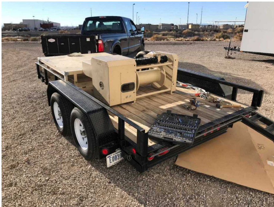
Trailer was outfitted with an old helium rack to add capability. Winch was mounted to the frame of the trailer and 4" U-channel was added to further secure the winch to the frame.
