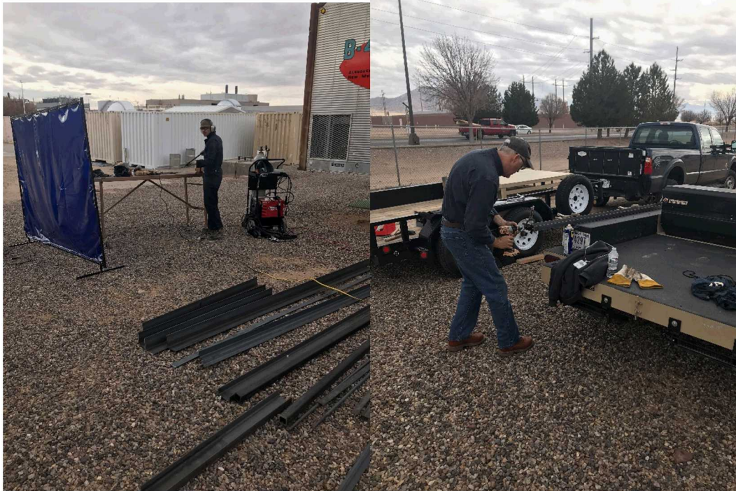
A new helium rack and U-channel crossmember being fabricated.
