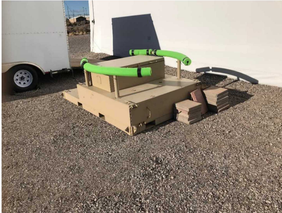
Old NM winch trailer electronics control box and mounting frame were removed to make the trailer user friendly.
