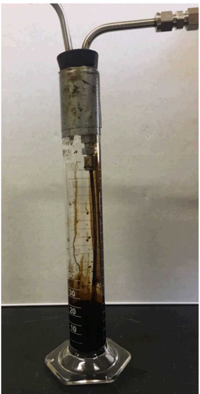
Fig 2.2.33: Photograph of outflow collection graduated cylinder for crude oil and subsequent gas displacement tests.
