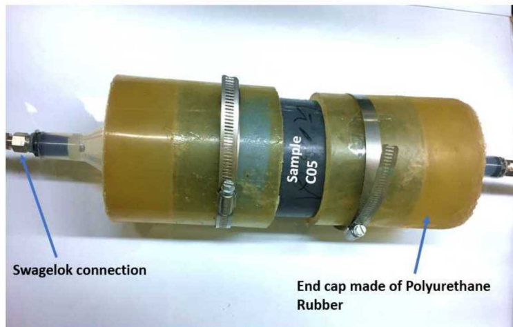
Fig. 2.1.18: Sample C05 for Gas permeability test (before epoxy intrusion).
