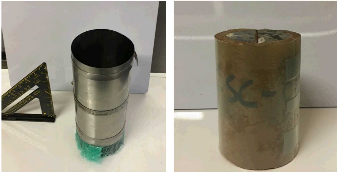
Fig. 2.1.9: (a) Left, a mold for Polyurethane Rubber Compounds PMC 770, and (b) right, completed Type 3 sample (CSC 02).
