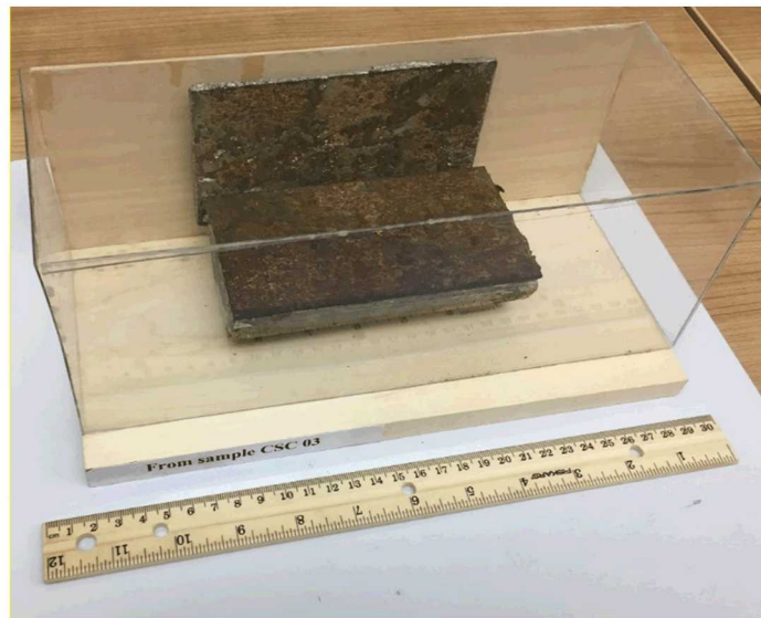
Fig. 2.1.12: Corroded plate with molded fusible alloy (Wood's metal) – sample CSC 03
