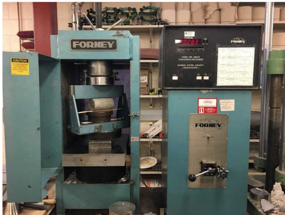
Fig. 2.1.2: Tensile splitting (Brazilian test) equipment. Cylindrical cement sample is in load frame on left, control system is on right.
