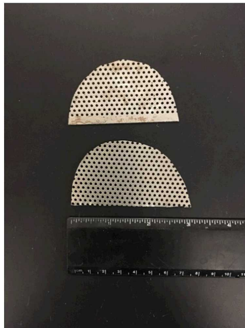
Fig. 2.1.4: Perforated thin steel sheets used to create offset of fractured cement samples.
