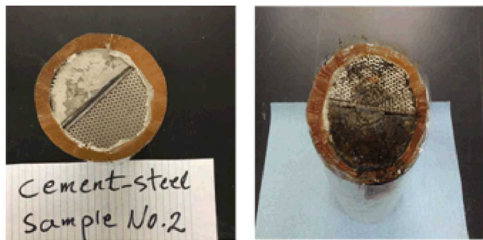
Fig 2.2.34: Pre-test (left) and post-test (right) photographs of the top of sample CS02 showing staining and accumulation of waxy deposits from crude oil.
