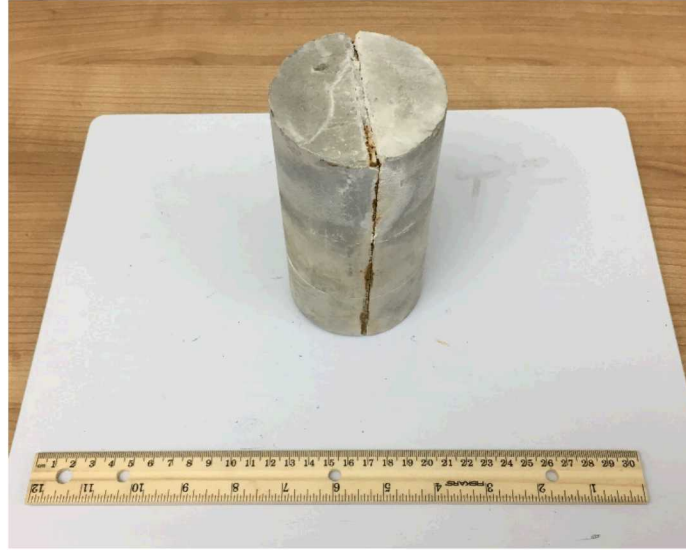
Fig. 2.1.11: Hardened cement paste (prepared from Zia Portland cement) with one-face protected hot rolled steel plate, after electrolysis (for sample CSC 04)
