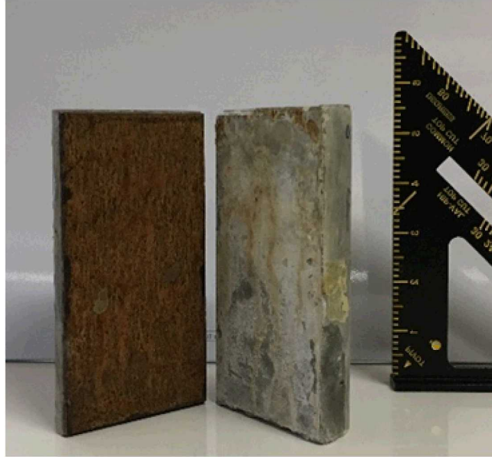
Fig. 2.1.8: Split cement sample with steel plate affixed to one cement face
