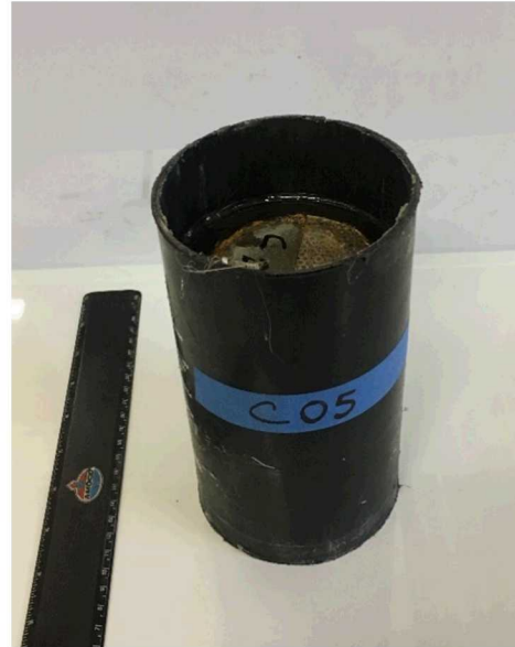
Fig. 2.1.17: a) Left, Schematic section of sample in enclosure, b) Right, Sample C05 in PVC enclosure.
