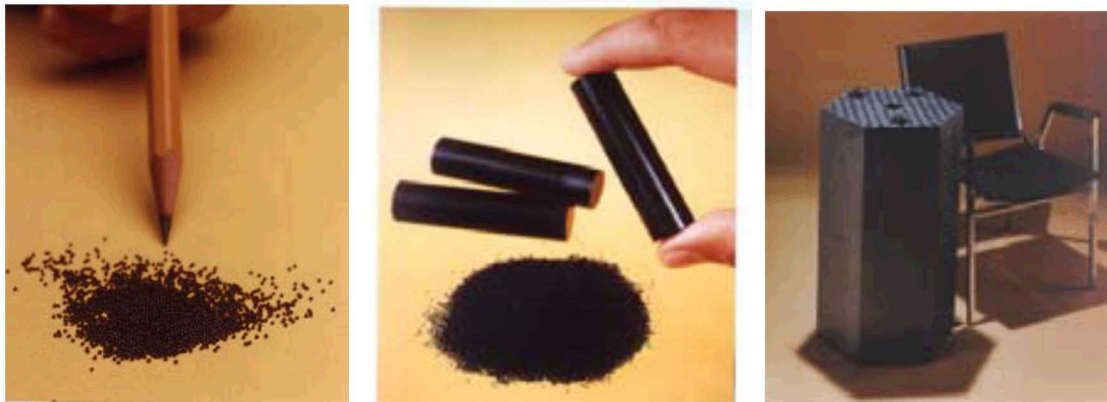
Figure 2. TRISO coated particles (left) are formed into fuel compacts (center) and inserted into graphite fuel elements (right). Taken from Sterbentz et al. [2004].
