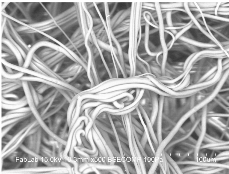
Figure 6 – An SEM micrograph of a nylon 6 fabric produced by the 3M Company.
