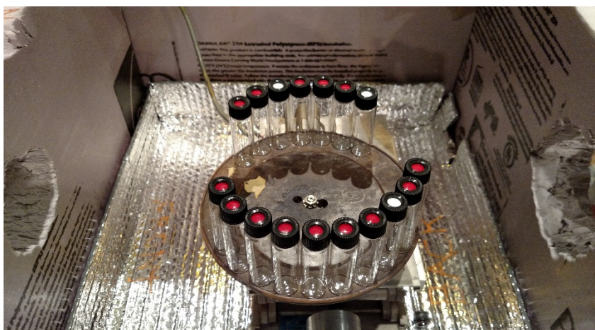
Figure 10 – The inside of the insulated irradiation chamber for controlling temperature during irradiations.
