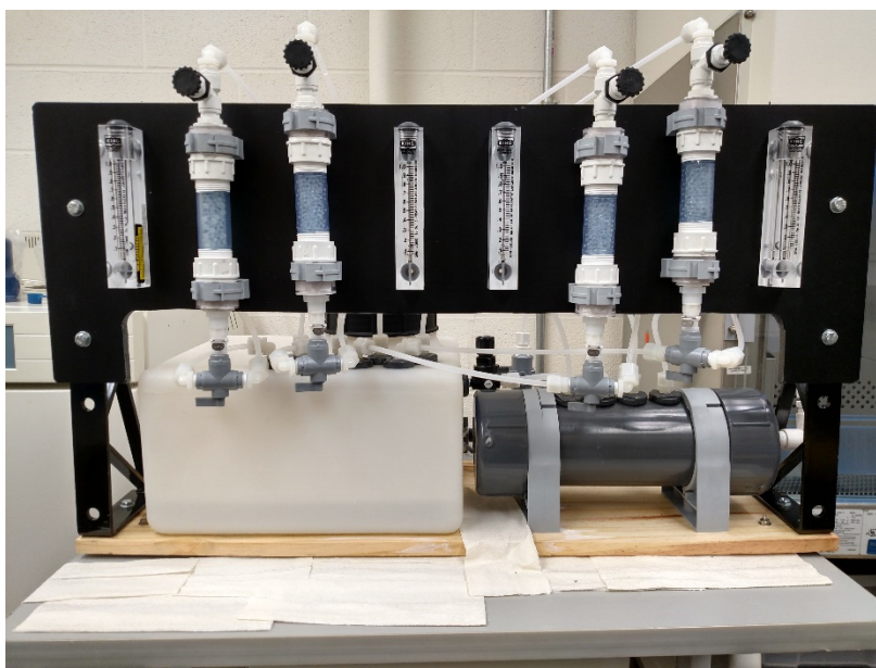
Figure 17 – The front view of the flow system designed to test fabrics under conditions similar to the testing performed at PNNL.
