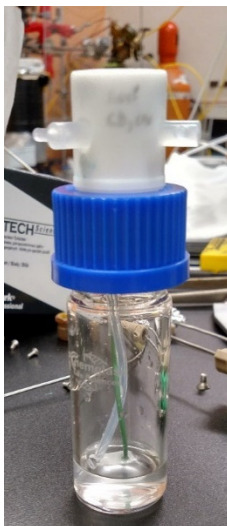
Figure 11 – The reservoir bottle from which monomer solution was drawn for Van de Graaff pulse radiolysis experiments. The cap of this bottle allows the solution to be sparged with a gas while sample is withdrawn using a syringe pump.
