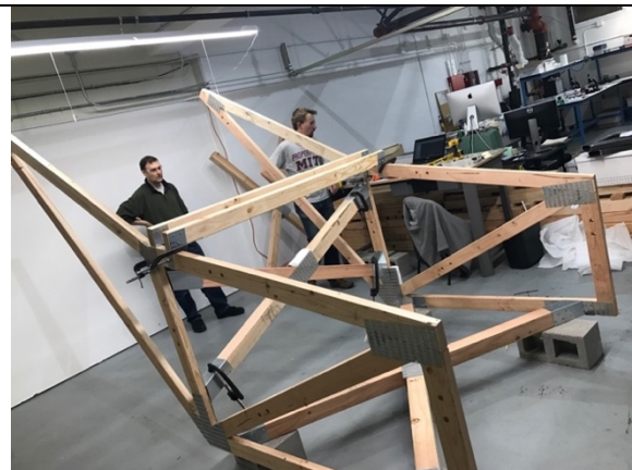
Lifting of the specimen to insert screws underneath trusses. Installation of lateral diagonal cross members
