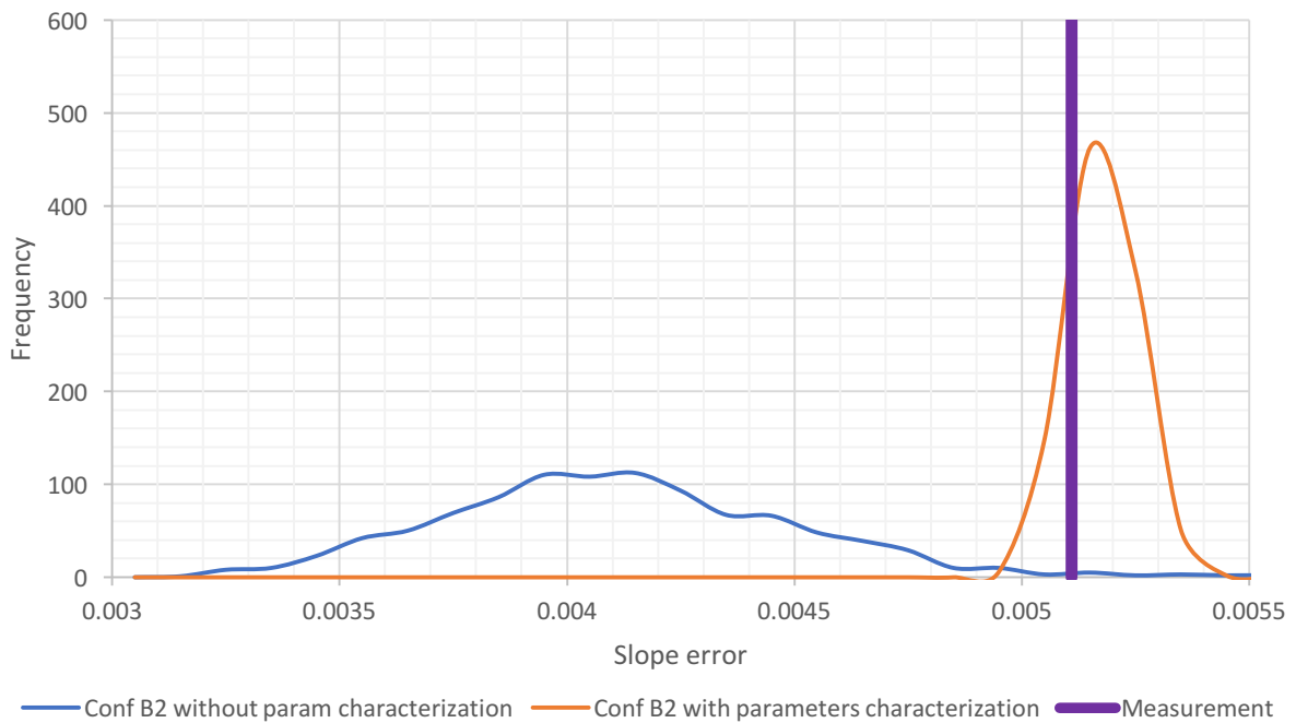
Figure 3-68. Slope error prediction for configuration B2. Comparison between original model with uncertain parameters and revised model with measured parameters.
