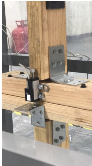
b) Diagonal member wood to wood screws
