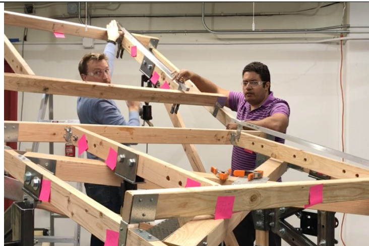
Alignment of mirror brackets using an alignment rod and laser tracker
