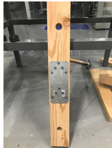
c) Diagonal member joints using metal tie plates
