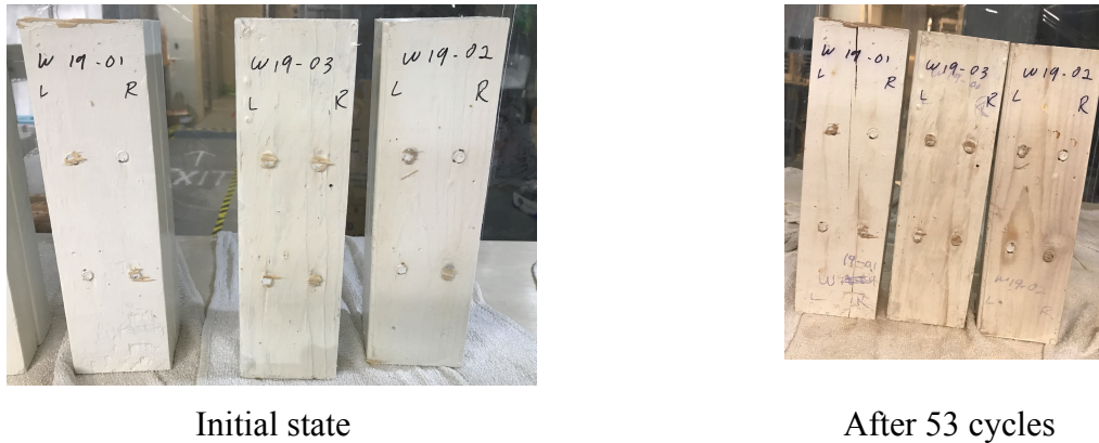
Figure 3-24. TimberLOK joints with 2 coats of LATEX paint
