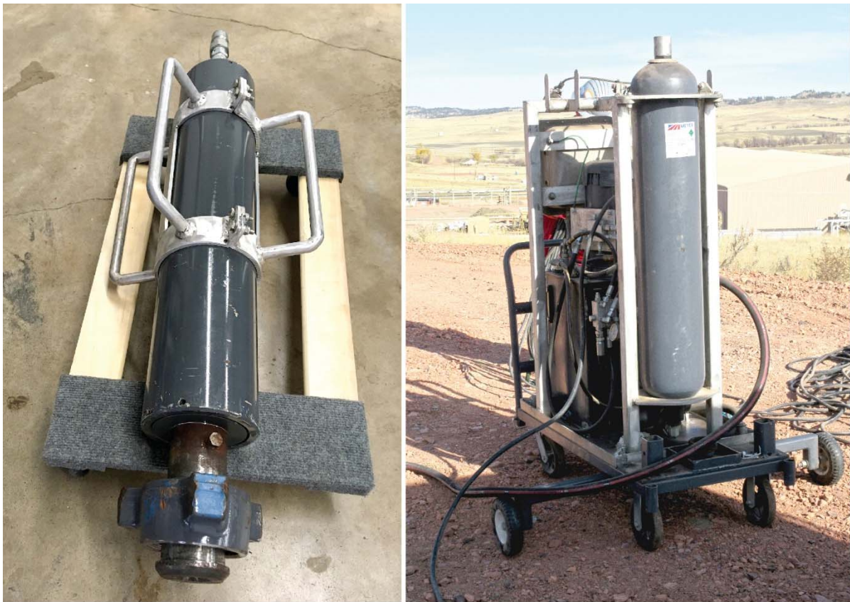
Figure 16. Left: the second-generation hydraulic “displacement” source. Right: source hydraulic power pack.
