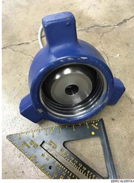
Figure 17. Second-generation hydrophone receiver for use on the source well. High-pressure pulses produced by the hydraulic displacement source required a more robust receiver design.
