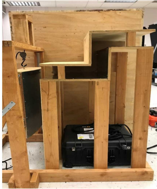
Figure 45. Ventilation channel mockup used for testing the robot/imager system.
