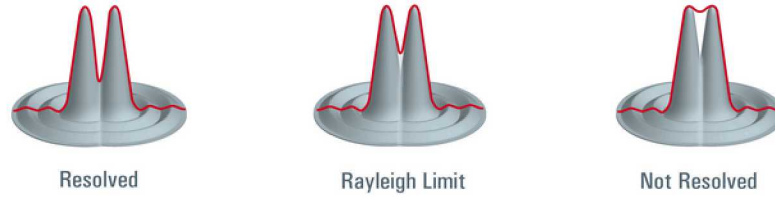
Figure 5. Example of two overlapping Airy disks and their spacing showing the resolved case; the Rayleigh limit of resolution, and the not resolved case.
