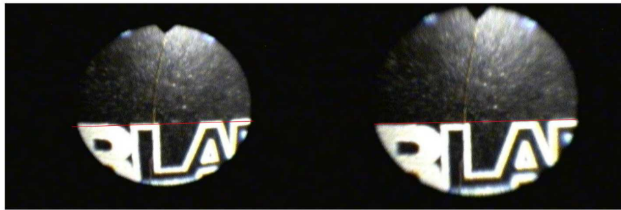
Figure 9. Photograph of lettering using the Hawkeye borescope. Left: barrel distortion is visible as curvature of the lettering. Right: following correction using the MatLab script (right image), the distortion is gone.
