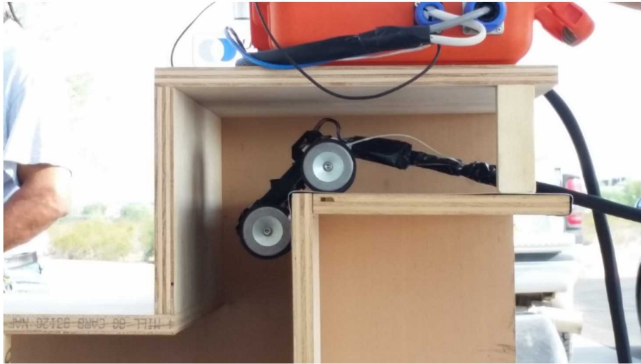
Figure 37. Magnetic Wheeled RTT robot traversing a mockup of a SNF dry storage system outlet vent.
