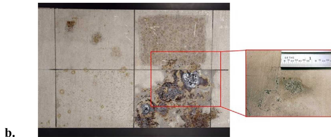
Figure 14. Four-point bend specimen. Apparatus design (a) and uncleaned and cleaned sample (b).
