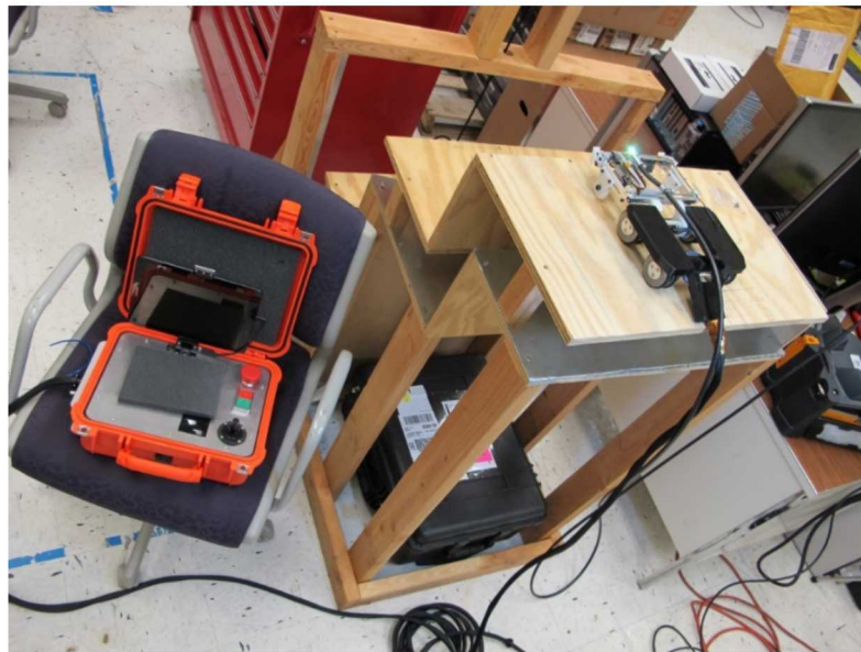
Figure 46. Images of the combined robot/imaging module traversing the storage system mockup.
