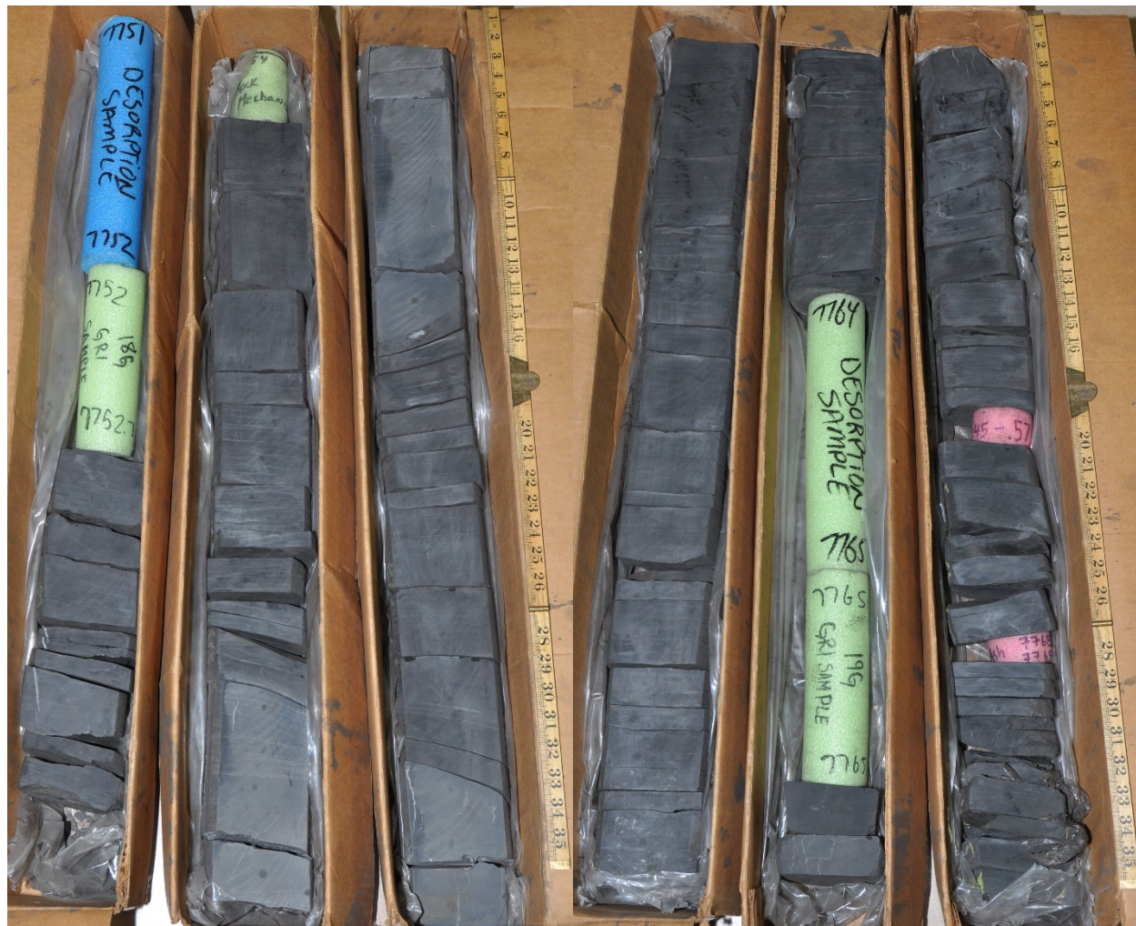
Figure 16: Armstrong #1 core photographs, from 7,751 to 7,769 ft.
