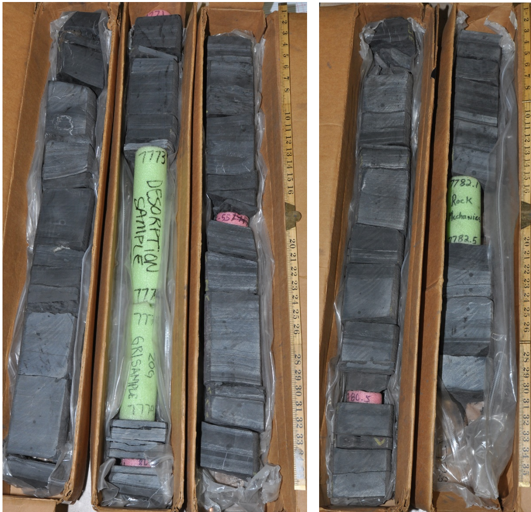
Figure 17: Armstrong #1 core photographs, from 7,769 to 7,783.4 ft.
