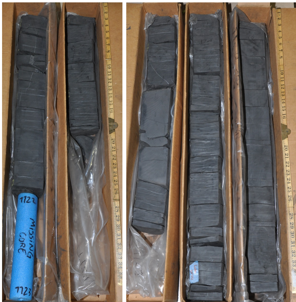
Figure 14: Armstrong #1 core photographs, from 7,720 to 7,732.9 ft.
