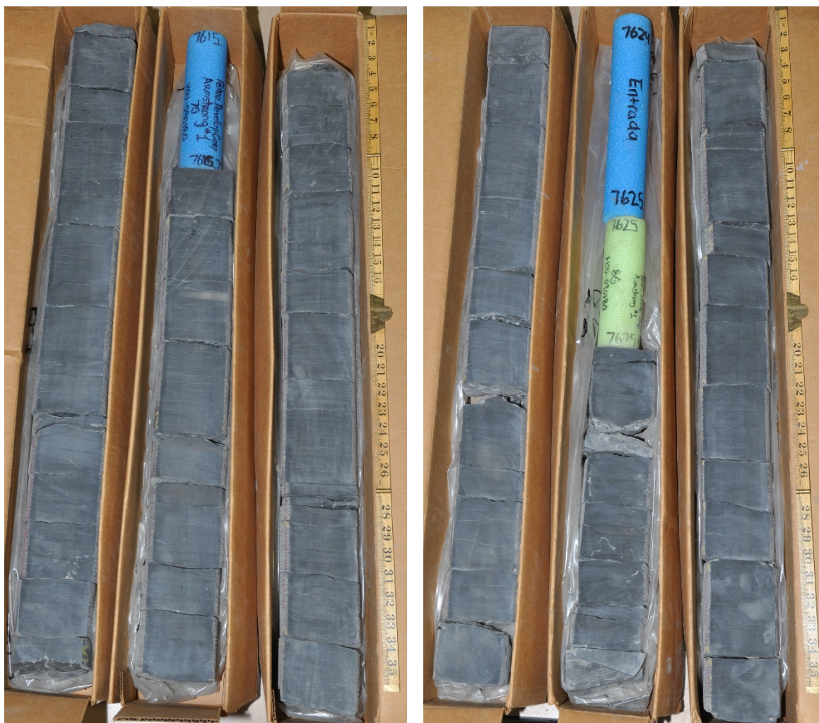
Figure 8: Armstrong #1 core photographs, from 7,612 to 7,630 ft.
