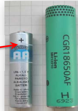
18650 cell format used in 85 kWh Tesla battery
