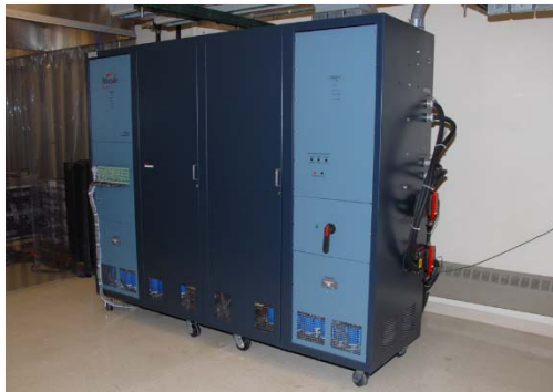
72 V 1000 A Bitrode (2 Channels)
