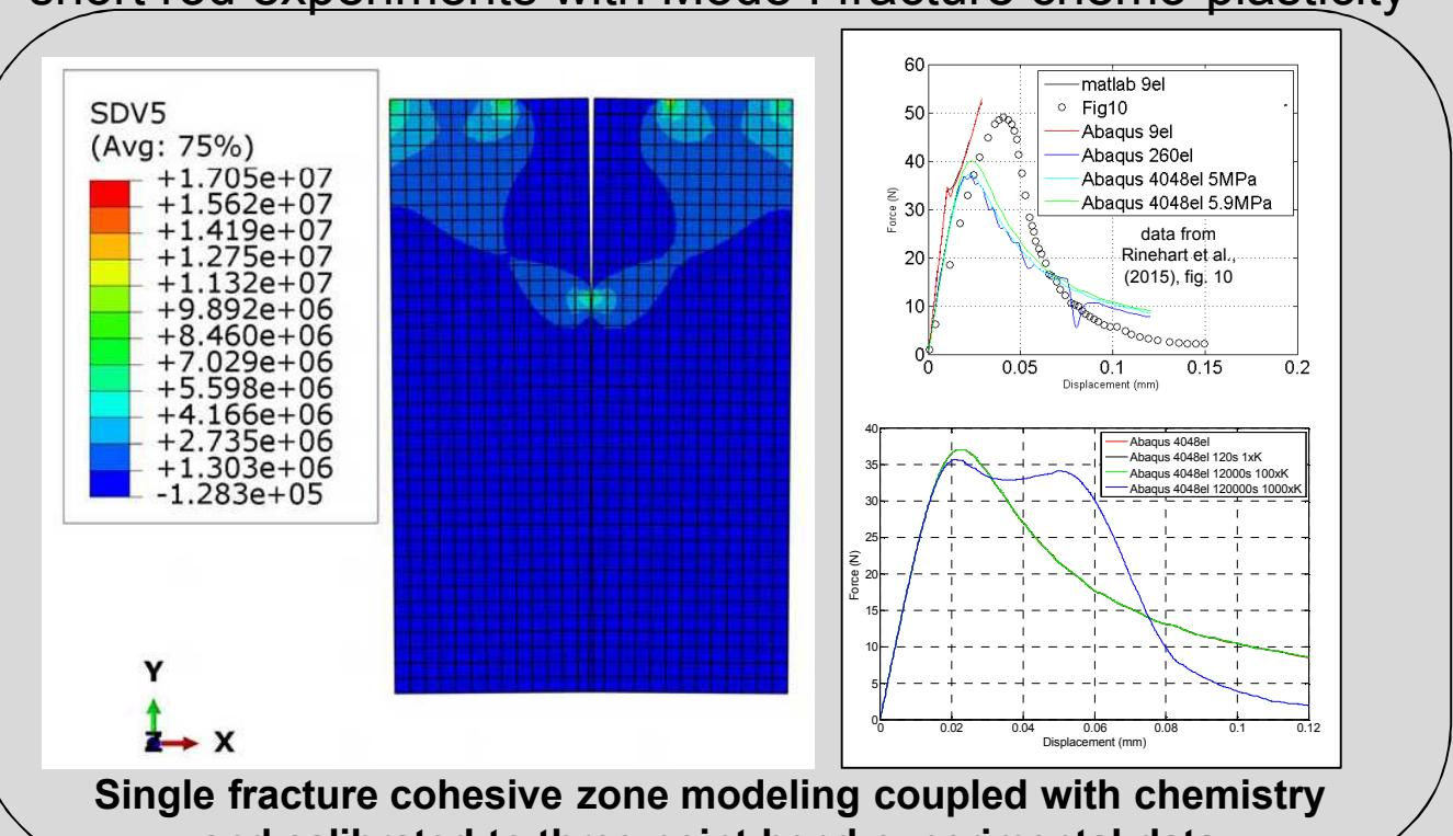
Single fracture cohesive zone modeling coupled with chemistry and calibrated to three-point-bend experimental data
