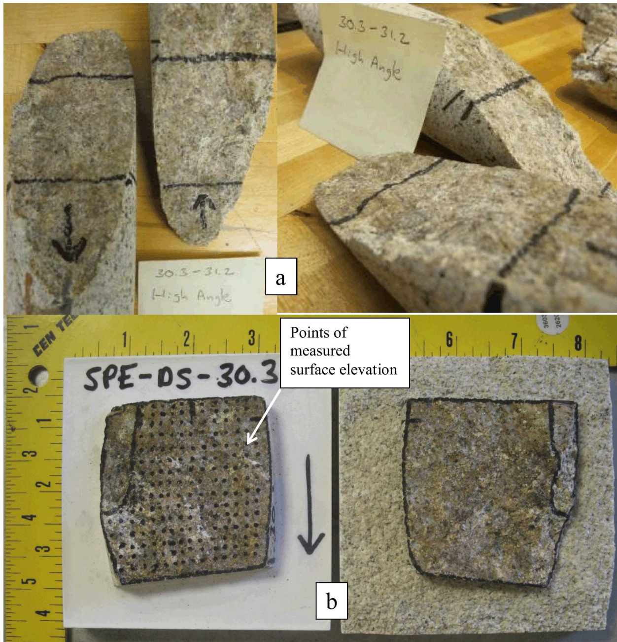
Figure 1: Specimen preparation steps for DS specimens: a) black lines on rock core indicate cut locations b) cut specimen supported in mold made from Plaster of Paris prior to placement in shear box.
