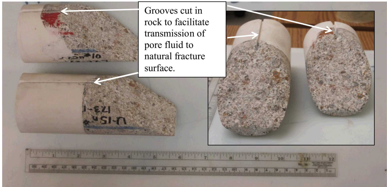
Figure 2: Specimen SPE2-FCT-17.4-52deg with ends filled with Plaster of Paris for mounting in pressure vessel.
