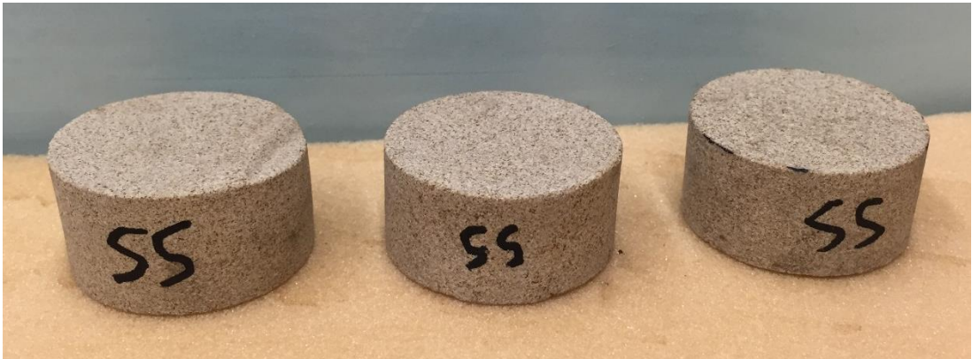
Figure 2.13. Sandstone samples for Brazilian test.
