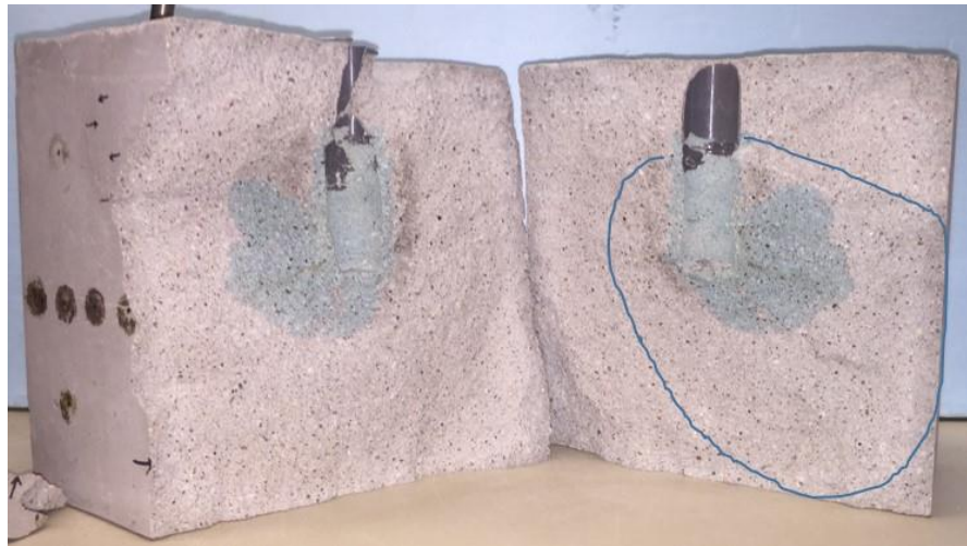
Figure 3.24: Internal fracture morphology of Sample 39 after dyeing and gas breakdown.
