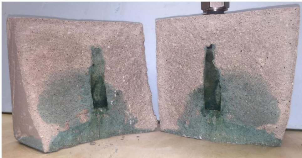
Figure 3.19: Internal fracture morphology of Sample 33 after dyeing and gas breakdown.
