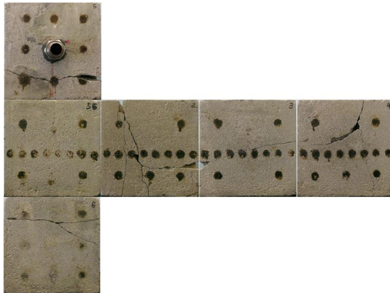
Figure 3.255. Surfaces of Sample 56 after dyeing and gas fracturing.
