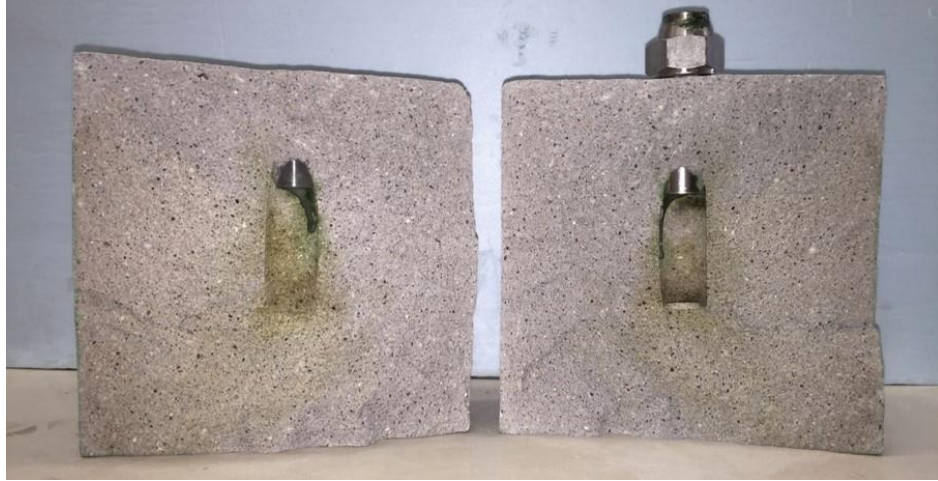
Figure 3.109. CO 2 injection induced fracture morphology of Sample 47.
