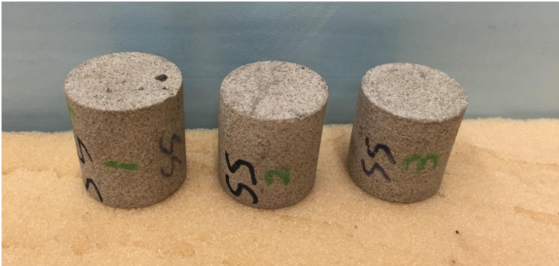
Figure 12. Sandstone core samples used for permeability and porosity measurement in CMS300.
