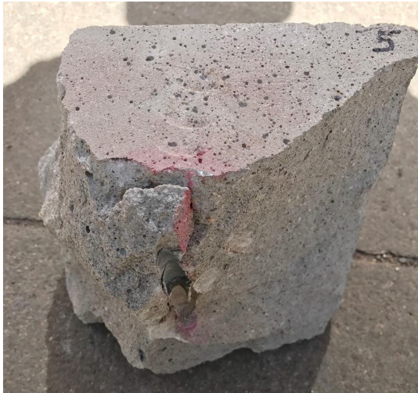
Figure 3.345: Water induced fracture that is perpendicular to y-direction in Sample 61.
