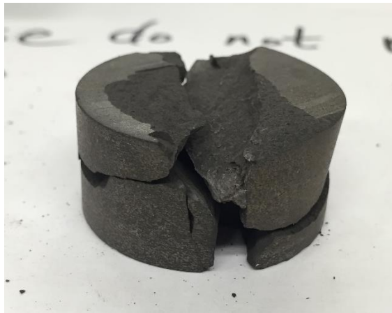
Figure 2.20. Shale sample SH-2 Br after Brazilian test.
