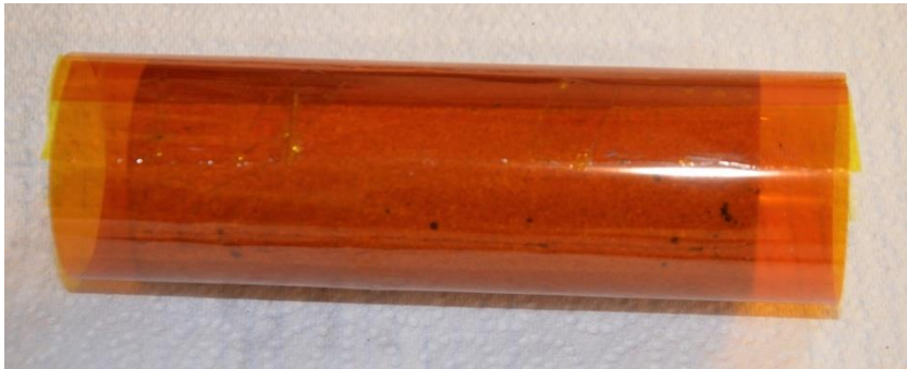
Figure 2.39. Nugget sandstone core wrapped in polyimide film.
