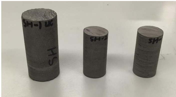
Figure 2.21. Shale samples for uniaxial compressional test.
