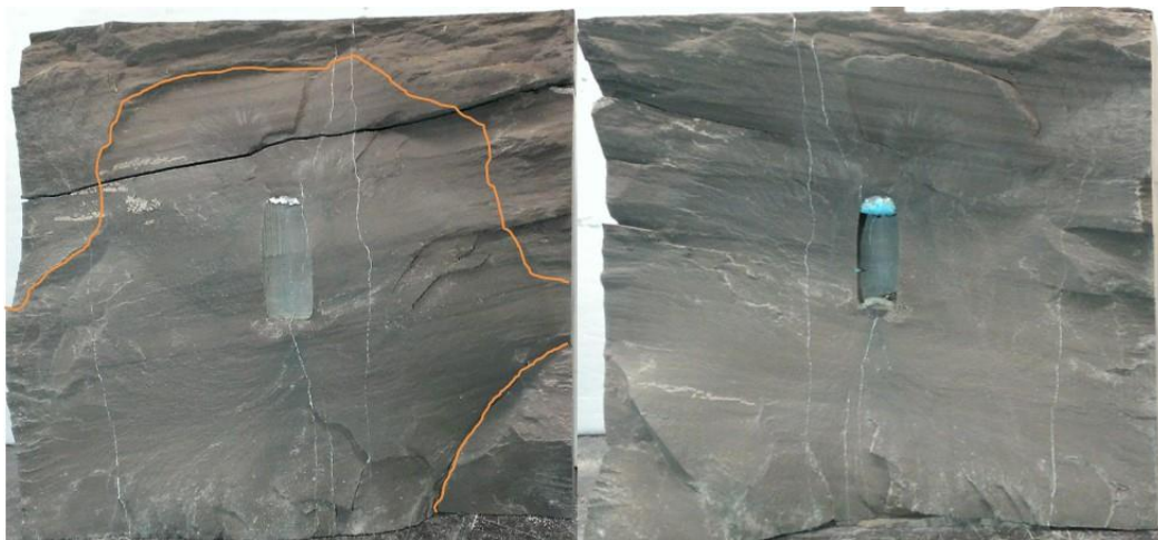
Figure 3.361. Sc-CO 2 injection induced fracture morphology of Shale Sample 1 after coloring and gas fracturing.
