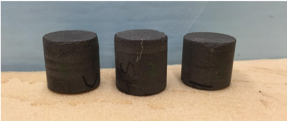
Figure 2.17. Shale core samples used for permeability and porosity measurement in CMS300.
