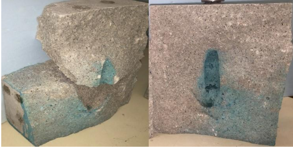
Figure 3.137. Injection induced fracture morphology of Sample 49 after dyeing and gas breakdown.
