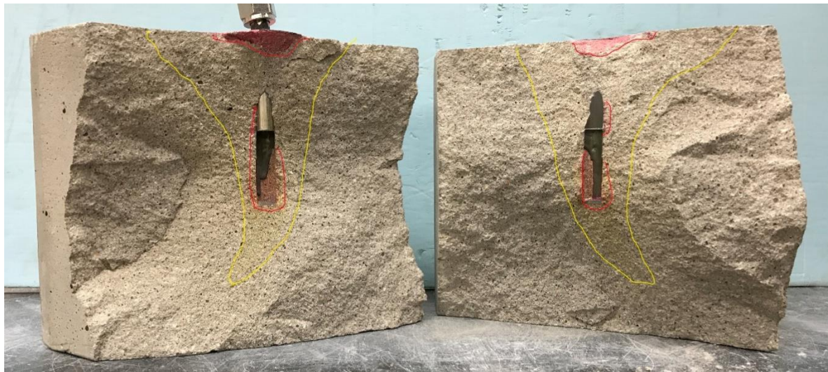
Figure 3.343: Colored water and CO 2 injection induced fracture planes in Sample 60.
