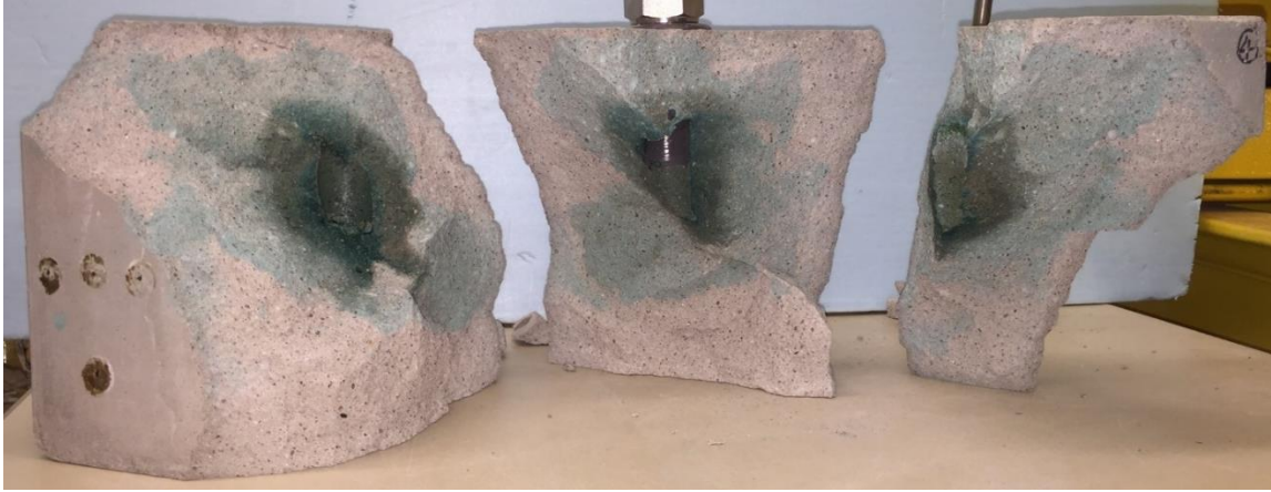
Figure 3.34: Internal fracture morphology of Sample 40 after dyeing and gas breakdown.
