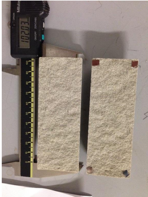
Figure 2.26. Split Gray Berea core with spacers.
