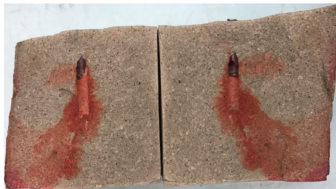
Figure 3.323. CO 2 injection induced fracture morphology of Sample 62 (opened from Surface 2).
