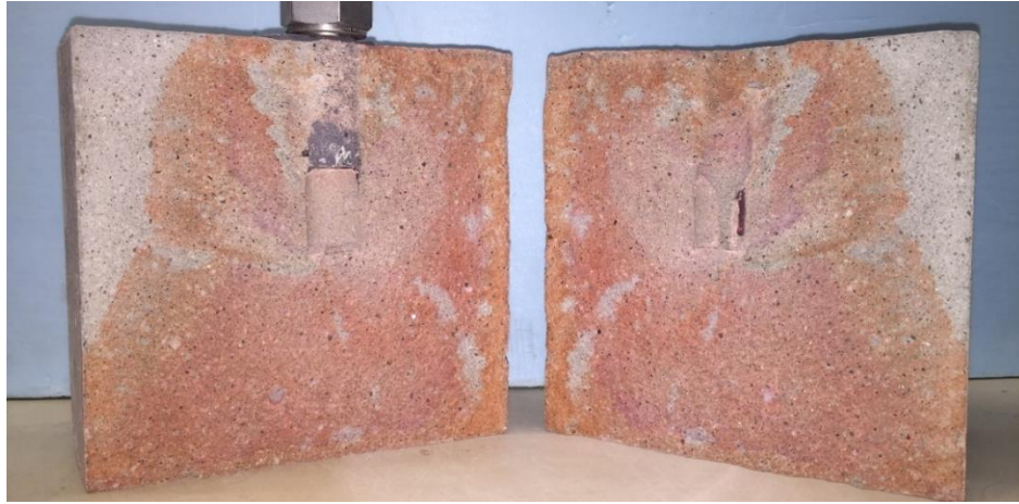
Figure 3.48: Fracture planes of Sample 27 after dyeing and gas breakdown.
