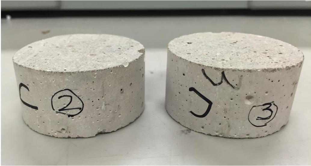
Figure 2.8. Concrete samples for Brazilian test.
