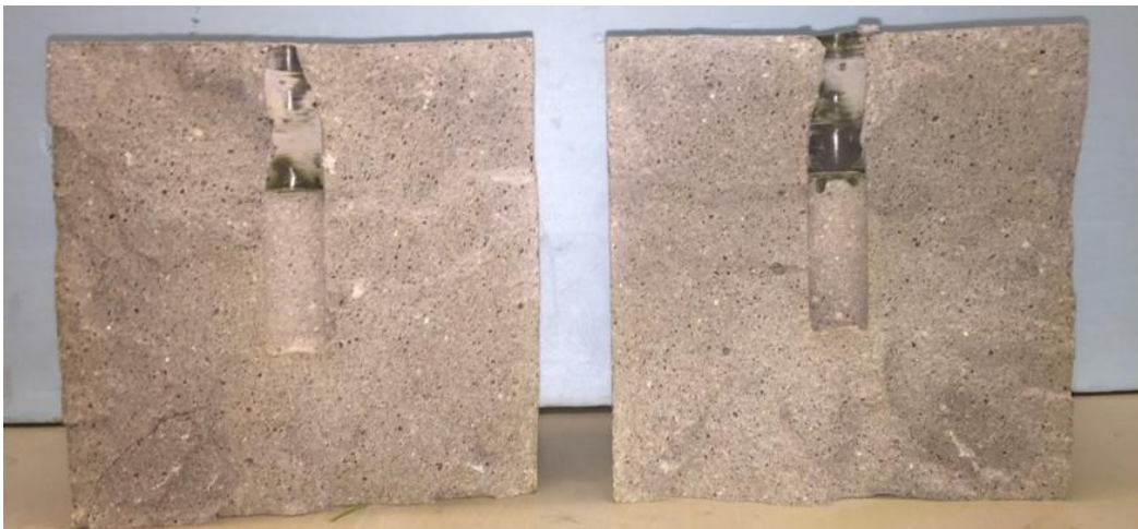
Figure 3.94. CO 2 injection induced fracture morphology of Sample 46 after gas fracturing.
