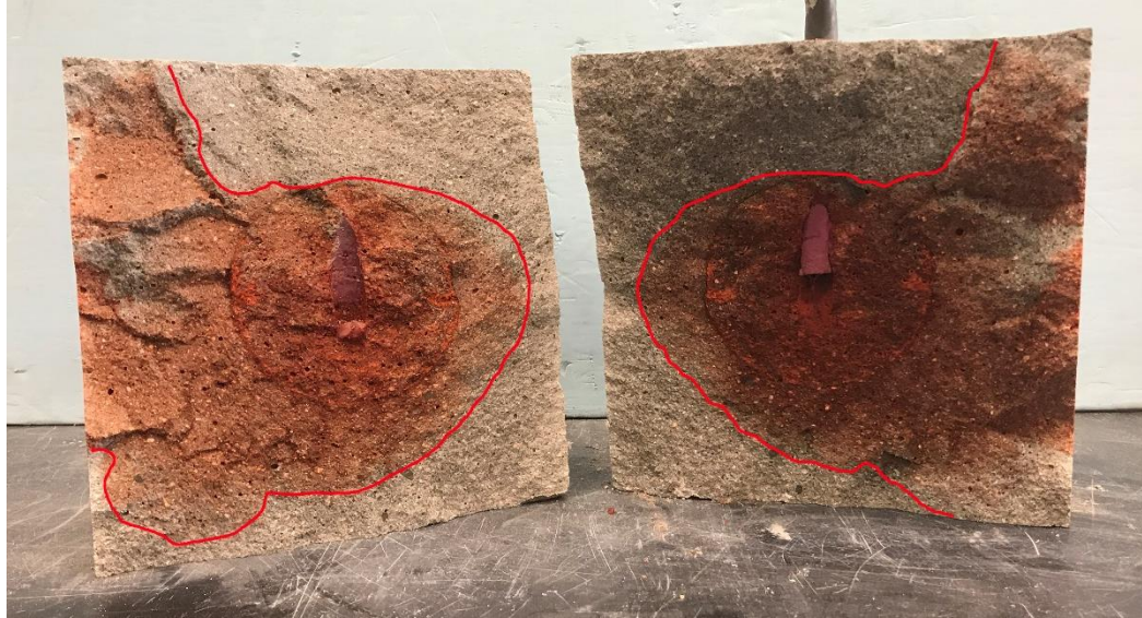
Figure 3.334: Colored CO 2 injection induced fracture planes in Sample 68. Note that the shape of high permeability ball is clearly distinguishable after dye injection.
