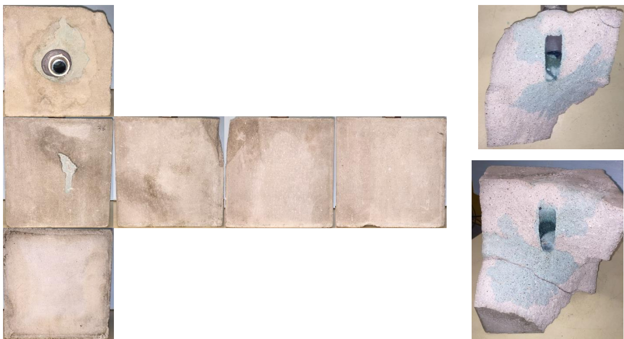
Figure 3.438: Fracture profile of Sample 38, with confining stress of 500-750-1000 psi. The left shows the outer surface of Sample 38 after fracturing. The right shows the fracture surface. Due to the low magnitude of confining stress and small stress differential, the fracture plane is relatively arbitrarily distributed.
