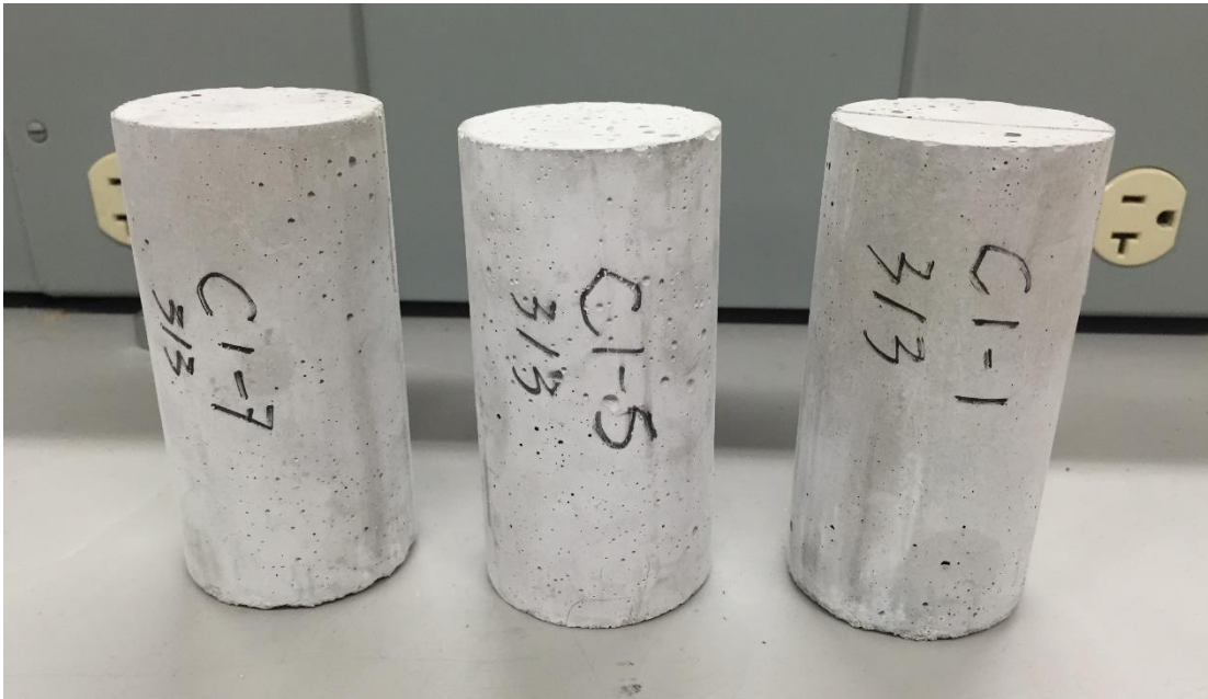
Figure 2.10. Concrete samples for uniaxial compression test.
