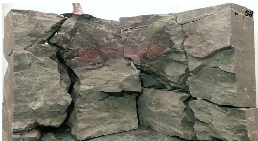
Figure 3.429. Slick water fracture morphology of Shale Sample 5 after gas break down.
