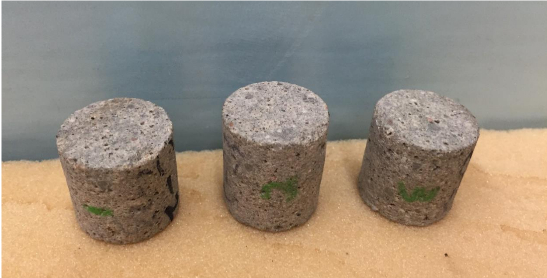
Figure 2.7. Concrete core samples used for permeability and porosity measurement in CMS300.
