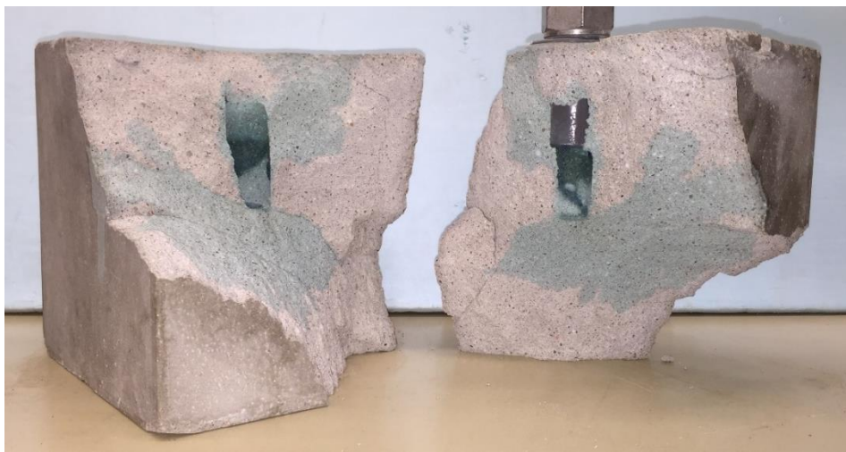
Figure 3.21: Internal fracture morphology of Sample 38 after dyeing and gas breakdown.
