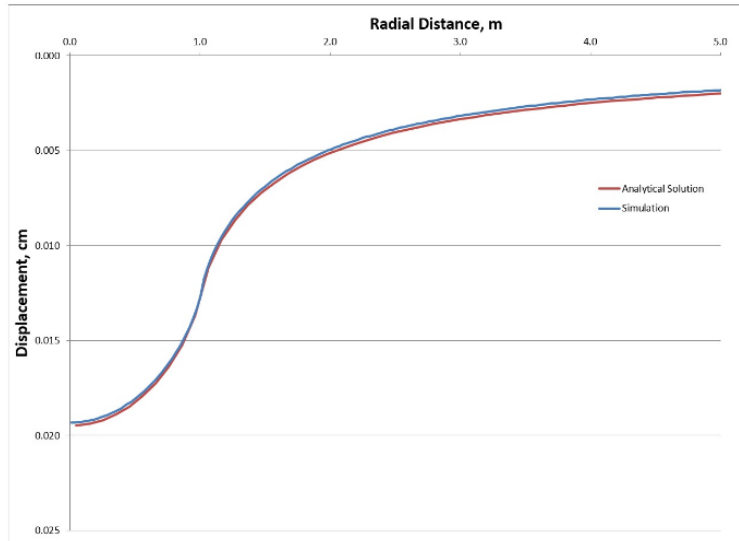
Figure 6.4. Analytical (solid line) and simulated (dotted line) displacements in rz-coordinates for semi-infinite medium subjected to circular load.
