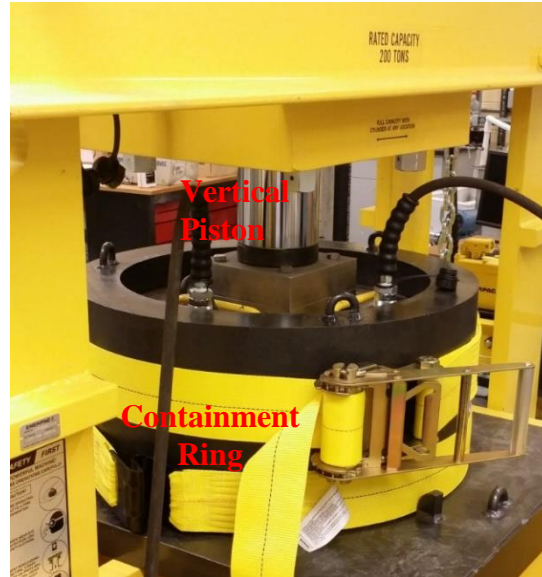
Figure 3.2: Vertical Piston on Rolling Frame and Containment Ring.
