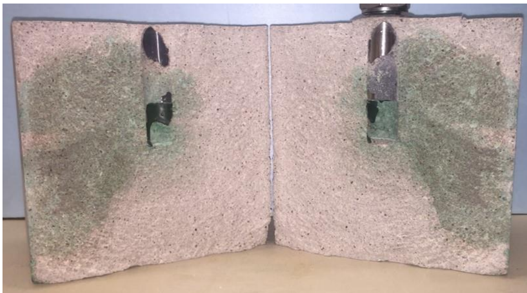
Figure 3.82. Colored CO 2 injection induced fracture planes in Sample 29.
