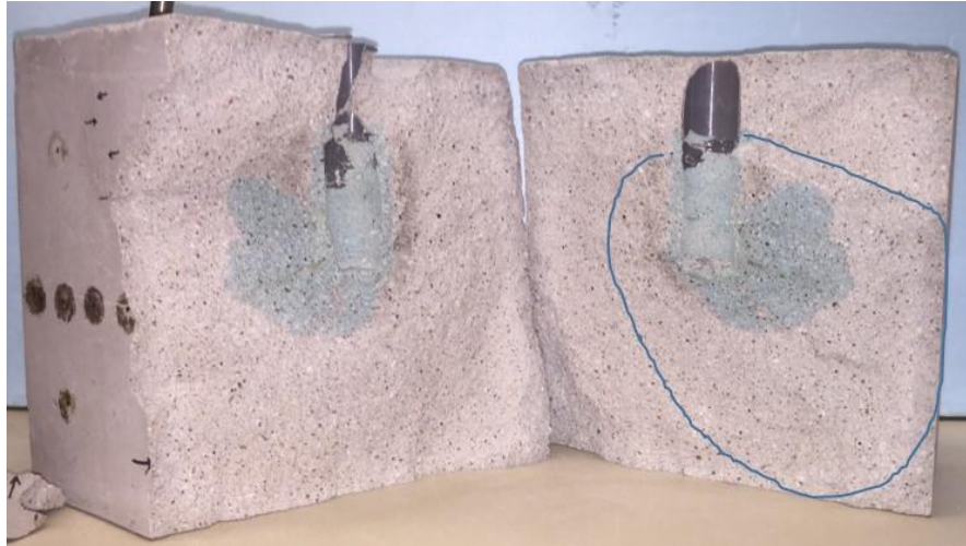
Figure 6.38. Internal fracture morphology of concrete sample after dyeing and gas breakdown.
