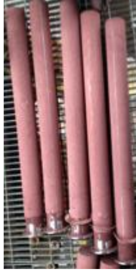
Figure 22. Secondary particle separator filter elements after Operation 2.
