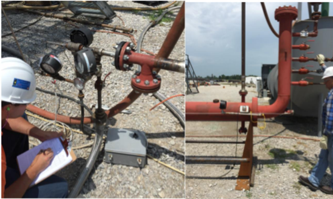
Figure 4. Factory acceptance test of raw gas burner in the simulated reactor chamber
