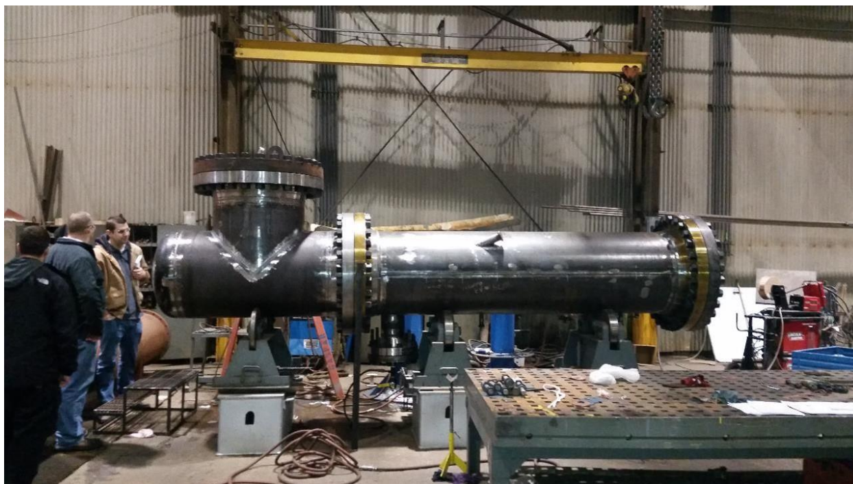
Figure 9. Picture of hydrotesting of burner chamber shell at Gaspar, Inc.
