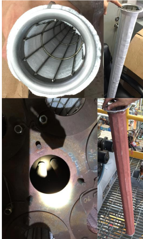
Figure 26. Photo of fabric filter elements prior to (top) and after (bottom) initial solid circulation testing.
