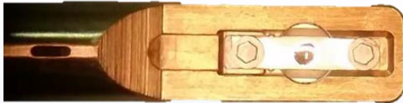
Traditional Gatan Heating and Straining Holder
