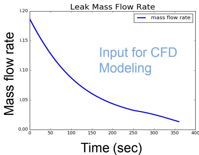
Calculates time required for tank to empty
