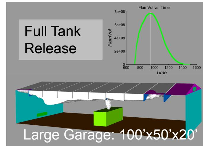
Results indicate that flammable concentrations can occur in regions not protected by NFPA 30A (lower than 18" from the ceiling).
