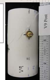
Sample printed vertical to loading direction (labelled with "H" ex: H9) vs. sample printed horizontal to loading direction (labelled with "V" ex: V9)
