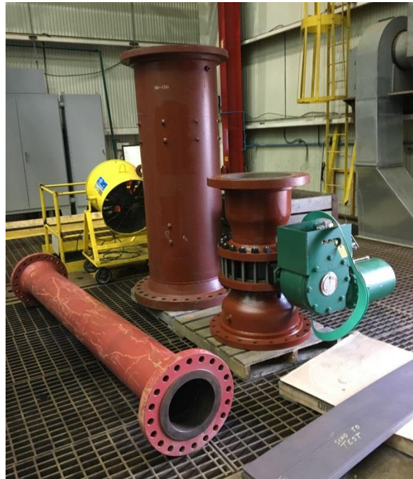
Figure 13 – Suction Line Instrumentation Spool; Discharge Piping and Discharge Throttling Valve
