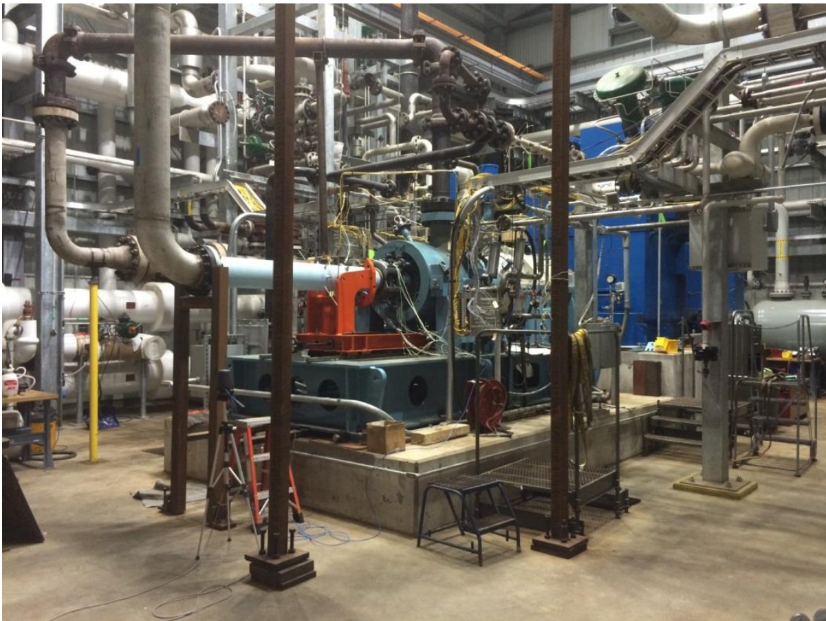
Figure 1 – DATUM S HP Compressor (DS-02-01) Installed in High Pressure CO 2 Facility
