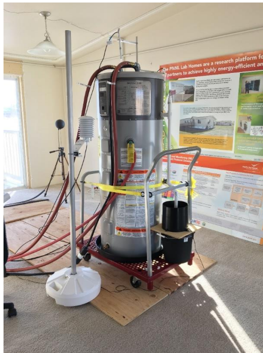
Figure 4.2. PNNL Lab Home B Experimental Apparatus Setup in the Living Room Location
