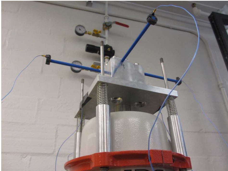
Figure 11. Shaker Test Setup Showing Gravity Off-Load Configuration
