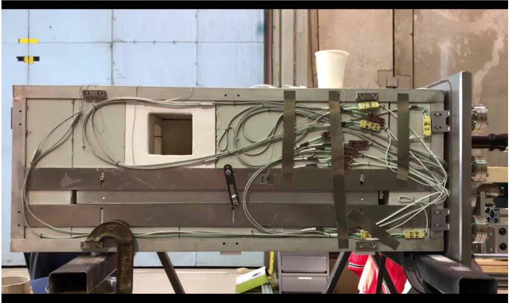
Ambient particle conveying test—side view of stick-slip plate action
