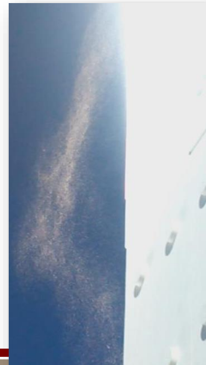
Particle loss from aperture during on-sun test
