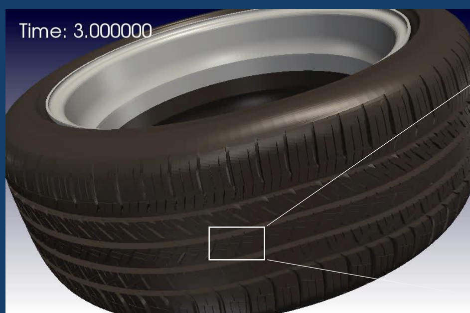
Finite element model of a Goodyear high performance tire being tested in extreme cornering maneuvers.
