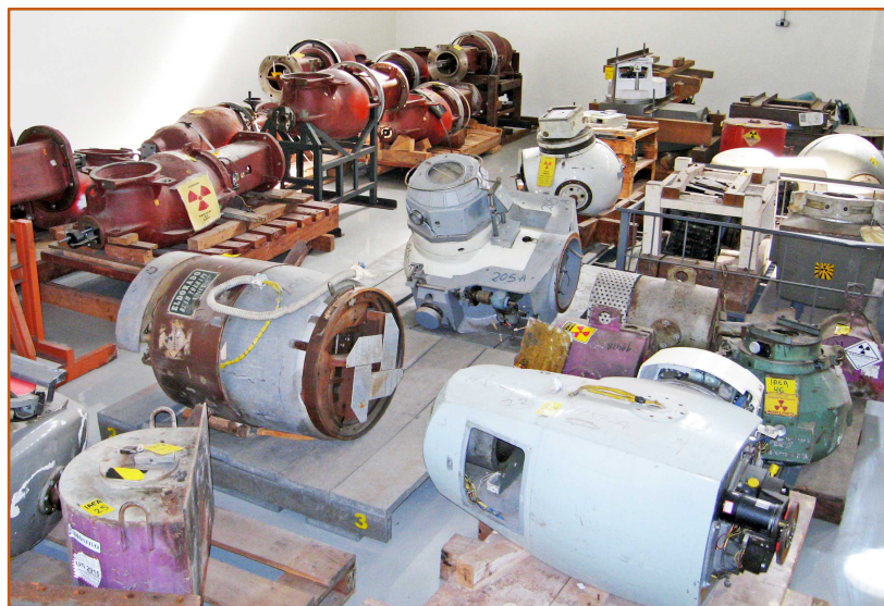
Fig. 2. Disused Medical “Source Devices” that Contain High-Activity DSRs
