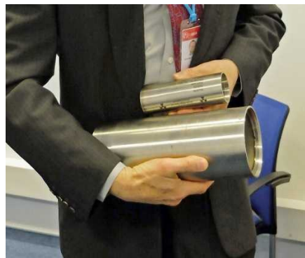
Fig. 5. Photograph of BDC Stainless Capsule and Container
