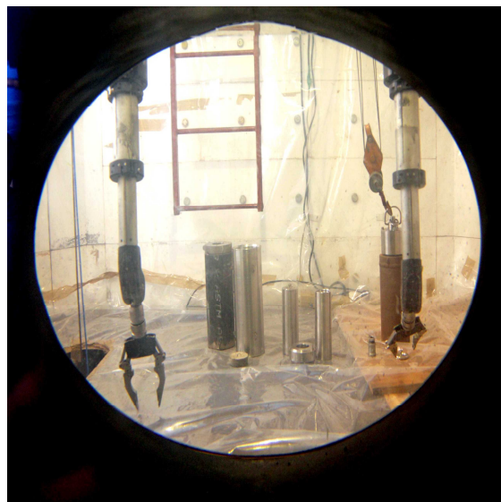
Fig. 9. View of BDC containers and capsules through 1.5 m thick window of mobile hot cell
