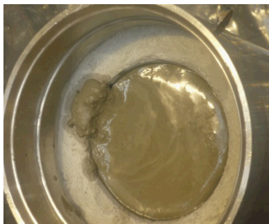
Fig. 12. Fresh Grout Filling the Opening of the Containment Barrier
