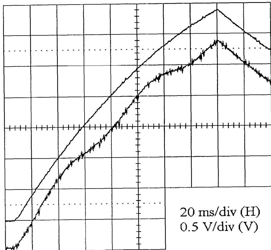
Figure 3 . Signals from the collector temperature monitor for rotation frequencies of 15 Hz (lower) and 600 Hz (upper).
