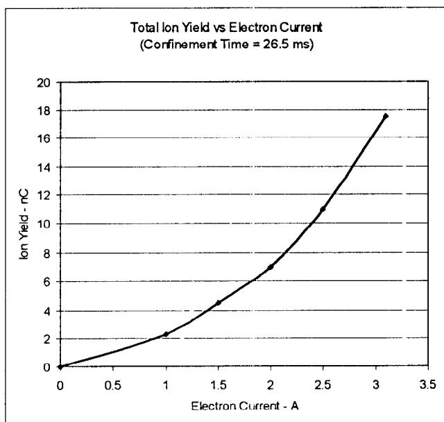
Figure 5 Total charge extracted for electron beam currents up to 3A.
