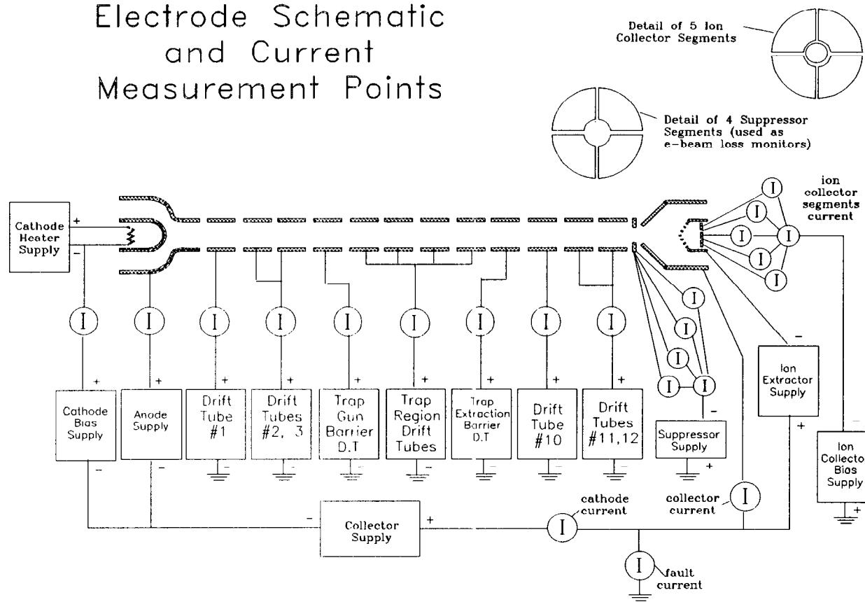
Figure 2: Electrode and current measuring schematic for electron and ion beam tests.
