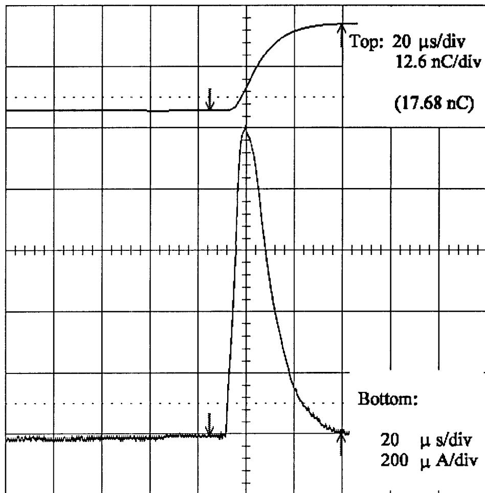
Figure 4 Trace of 1 mA ion pulse, produced by a 3A electron beam. The Total collected charge is about 17.5 nC
