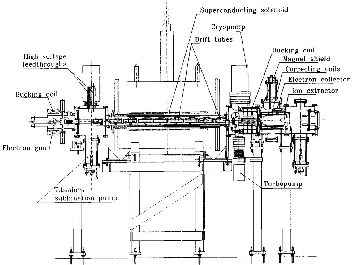
Figure 1: Layout of the electron beam test stand
