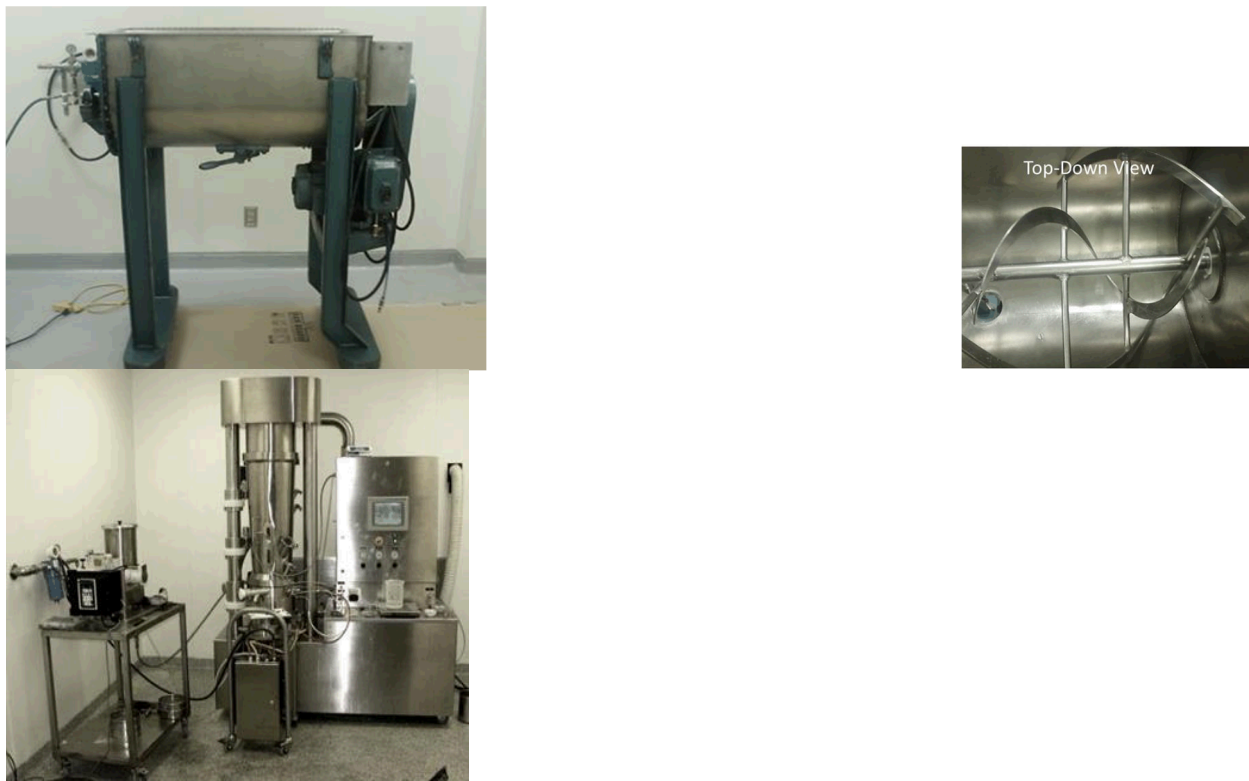
Figure 3: Left – ribbon blender; center – inside ribbon blender; right – granulator
