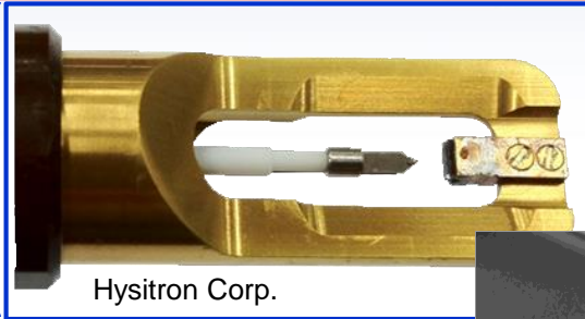
Hysitron PI95 In Situ Nanoindentation TEM Holder
