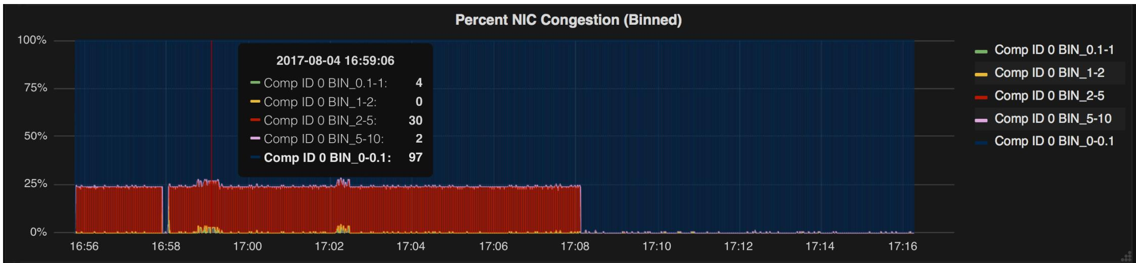
*Runtime analysis and visualization of shared network congestion metrics. Backpressure in the network due to multiple applications' traffic limits the injection rate, reducing application performance. Shown: Percentage of NIC's with performance-impacting values.*
