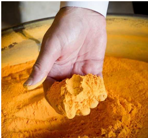
Yellowcake Uranium ( \text{U}_3\text{O}_8 ) Photo: Ivan Pierre Aguirre/Texas Tribune
