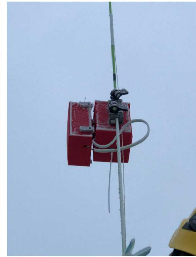
(a) POPS and iMet configuration. (b) Sky conditions at 23:55 when (c) Icing on tether, iMet, SLWC altitude record of 1.44 km was achieved. Tether is neon green when not covered in ice.
