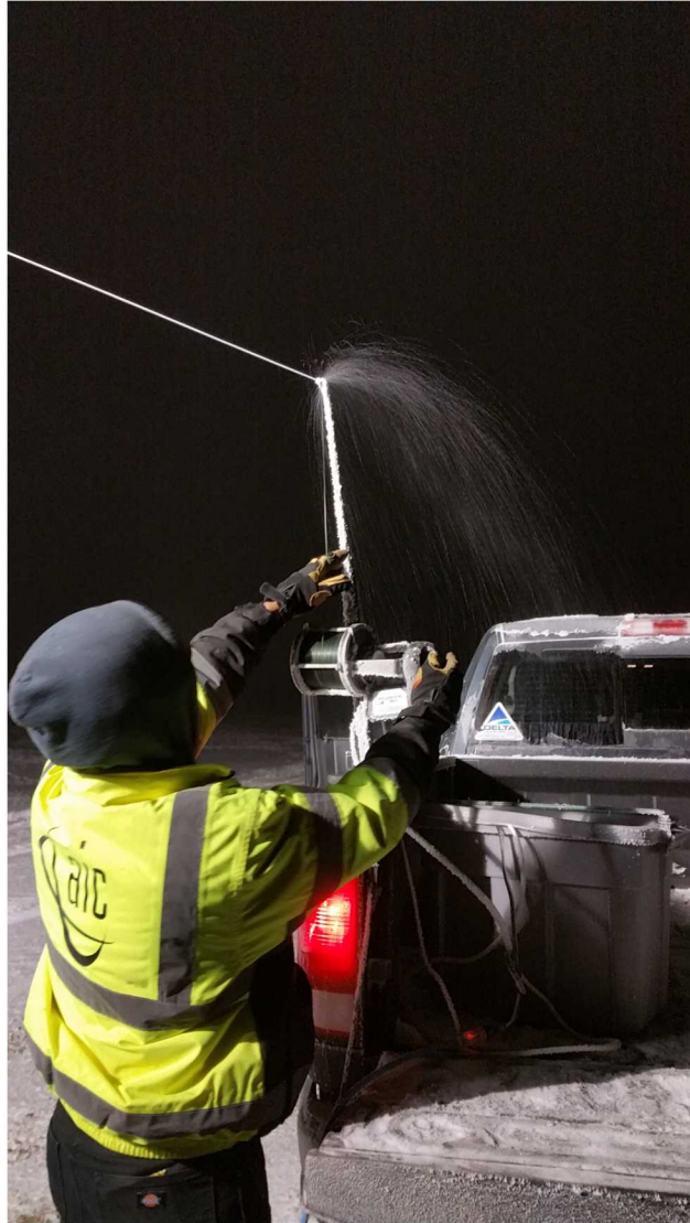
Figure 3.14. Deicing the tether going into the auto-reeler from the balloon on 15 November 2016.
