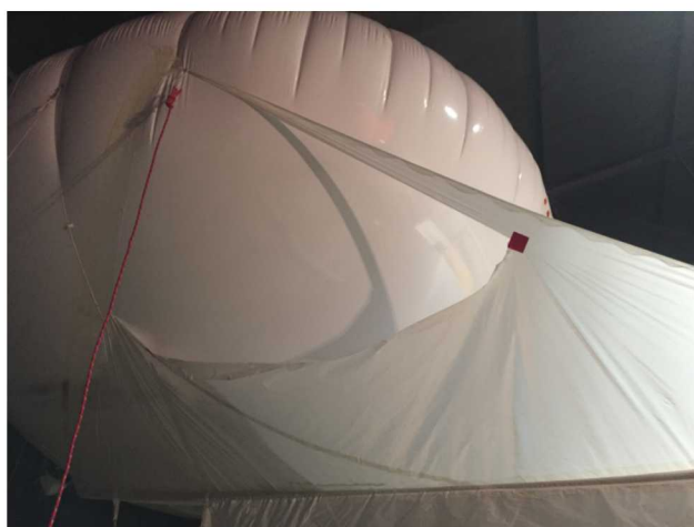
Figure 3.9. Torn helikite skirt, October 2016.
