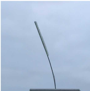
(d) Ice build-up on vibrating wire of SLWC. (e) Snapshot of computer logging (f) Initial SLWC data and tether raw frequency data in the vehicle ersonde SLWC from 13 October during TBS deployment of SLWCs. 2017. Panel plots from bottoms to Notice the depression of SLWC top are raw frequency, temperature, wire frequency upon entry into wind speed, and calculated concentration of supercooled liquid water when the sensor exits the cloud top. content as a function of time.
