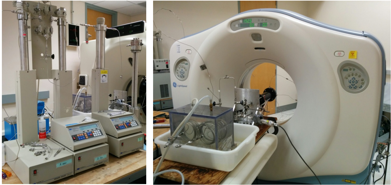
Figure 2.4: On the left image, and from left to right, double water pump, back pressure pump and two phase separator. On the right one, the core-holder inside the medical X-ray CT scanner and the gas-liquid flux heater box.
