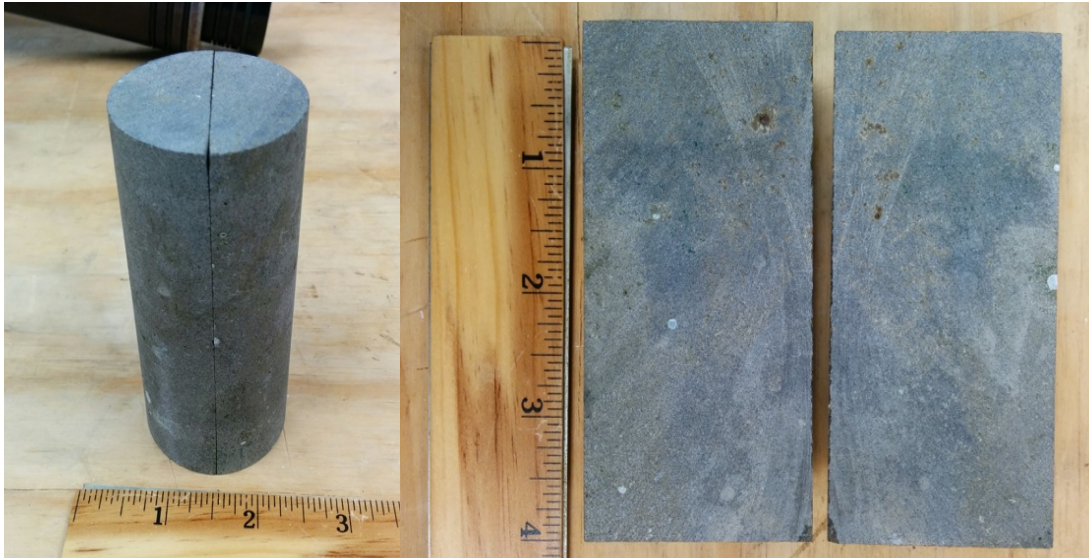
Figure 2.2: Basalt core with a saw-cut fracture. The two surfaces can be seen on the right image.
