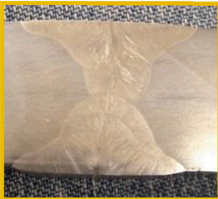
Photo of dry canister weld. Photo: SNL
