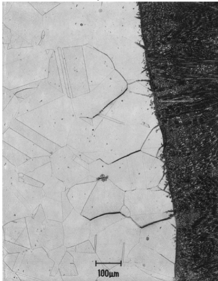
Inconel 718 HAZ liquation cracks; 43 ppm B
