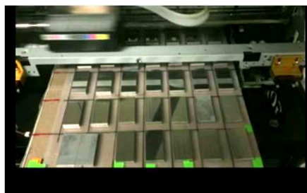
Inkjet printing for high-throughput salt loading
