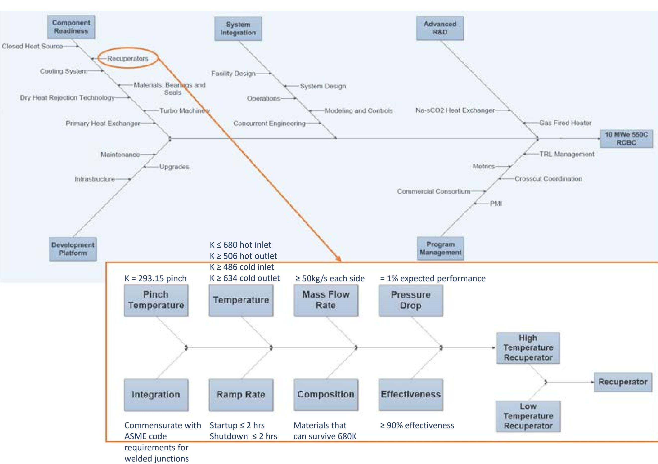
The System TRL can only be as high as the lowest component TRL and its interactions.
