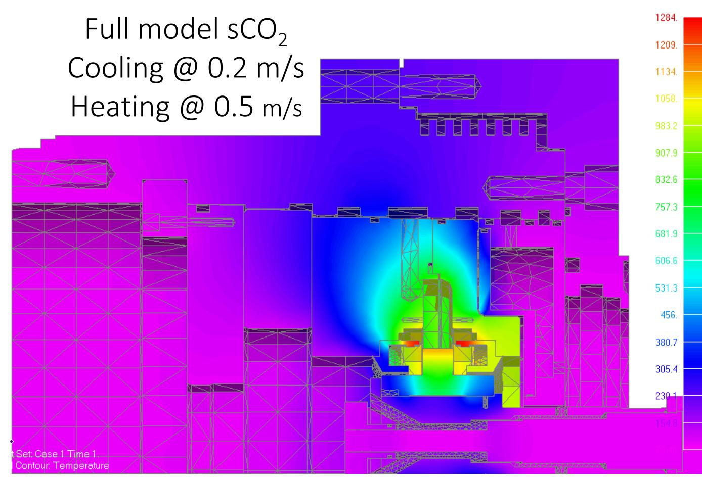
Full model sCO<sub>2</sub> Cooling @ 0.2 m/s Heating @ 0.5 m/s
