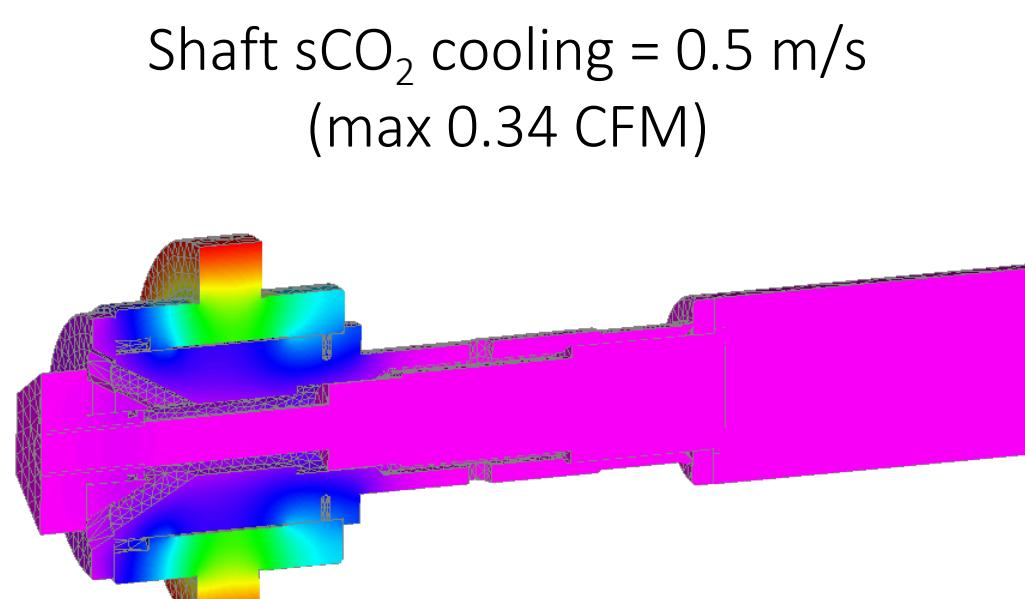
Shaft sCO<sub>2</sub> cooling = 0.5 m/s (max 0.34 CFM)
