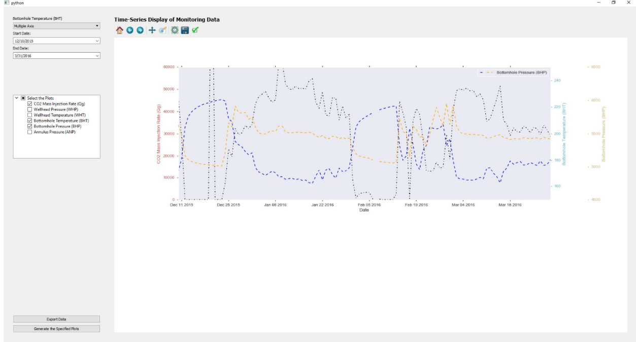
Figure 15. Module 1 multiple-axis plot option showing Qg, BHT, and BHP versus time.
