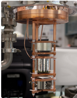
Fig. 2. Left: multi-detector system ( string ) including the copper mounts and cabling length of the MAJORANA DEMONSTRATOR. Right: noise curve of front-end operated in a string as a function of shaping time.
