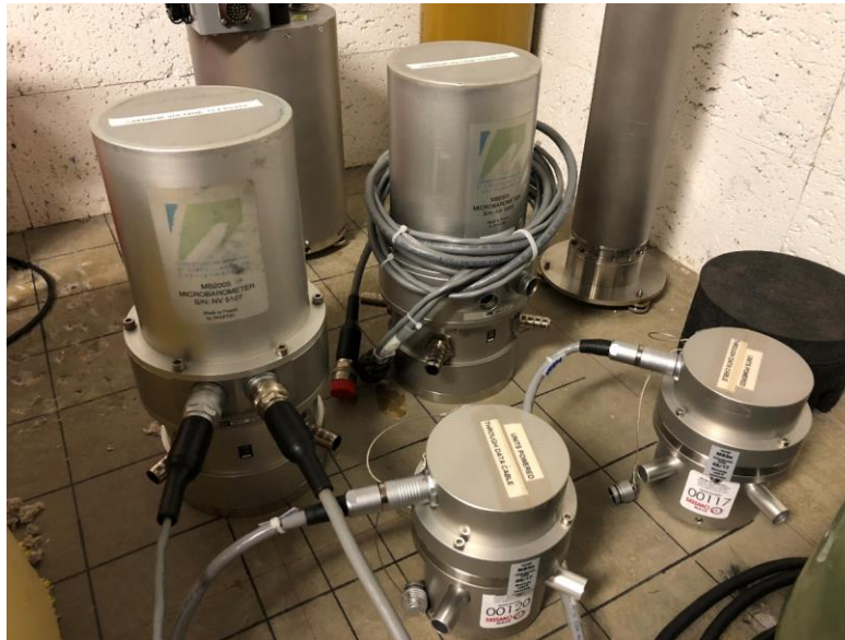
Figure 143 Centaur 5002 and MB3a infrasound sensor
