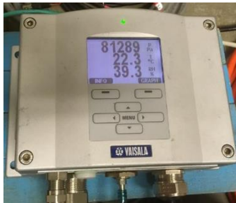
Figure 5 Vaisala Temperature Monitor within FACT Bunker
