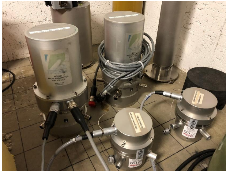
Figure 150 MB2005 infrasound sensor
