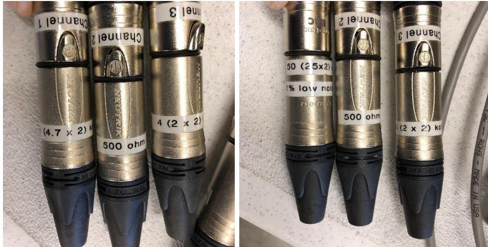
Figure 54 Temperature Self Noise Configuration Picture
