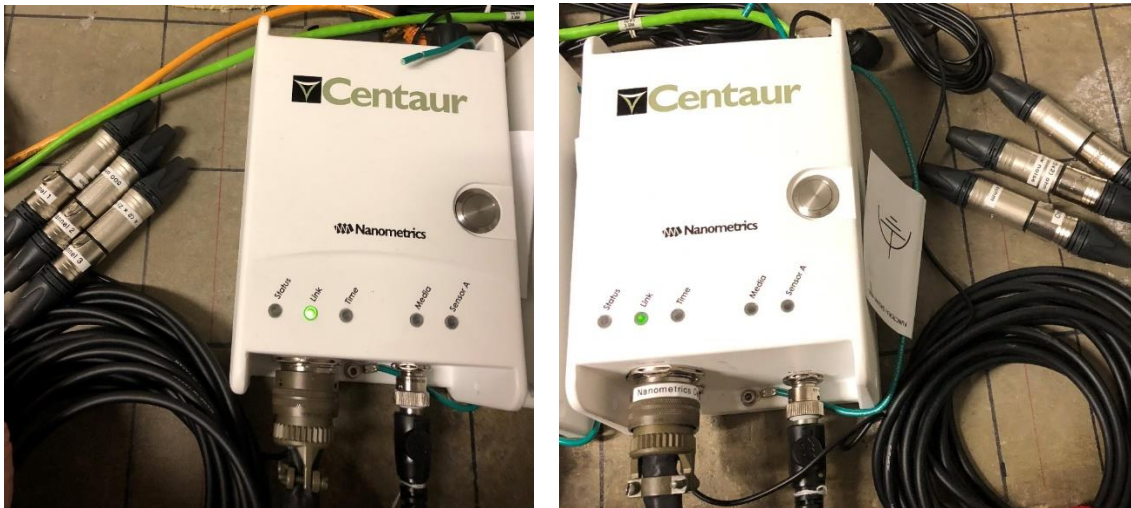
Figure 24 Input Shorted Offset Configuration Picture
