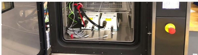
Figure 52 Temperature Self Noise Configuration Diagram
