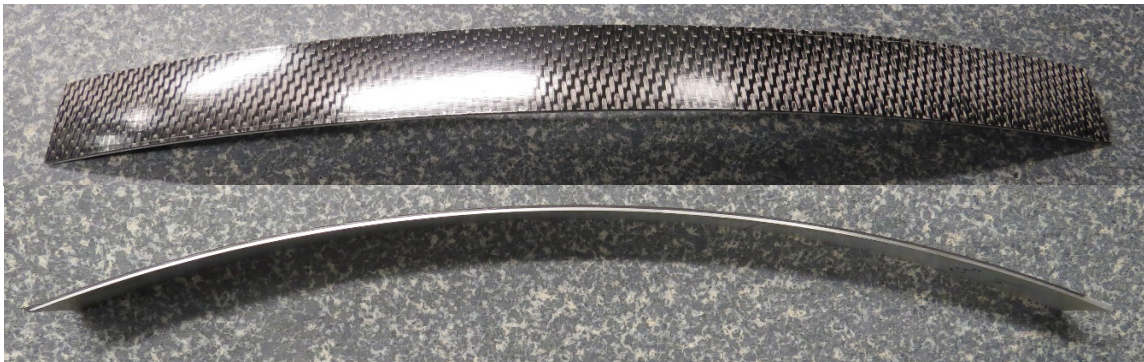
Figure 2.1: Manufactured bi-material strip
