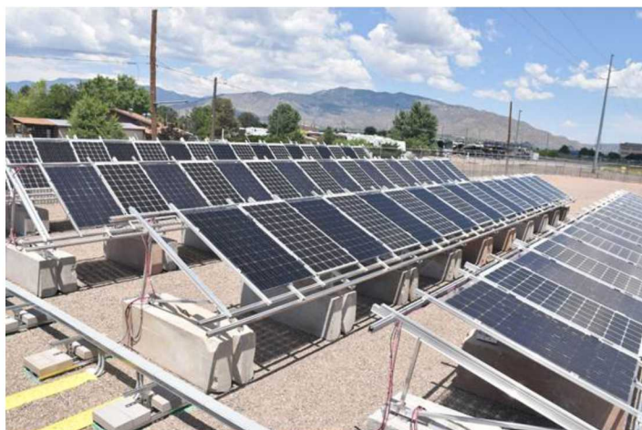
Fig. 3. Fixed-tilt, string level bifacial testbed at Sandia.
