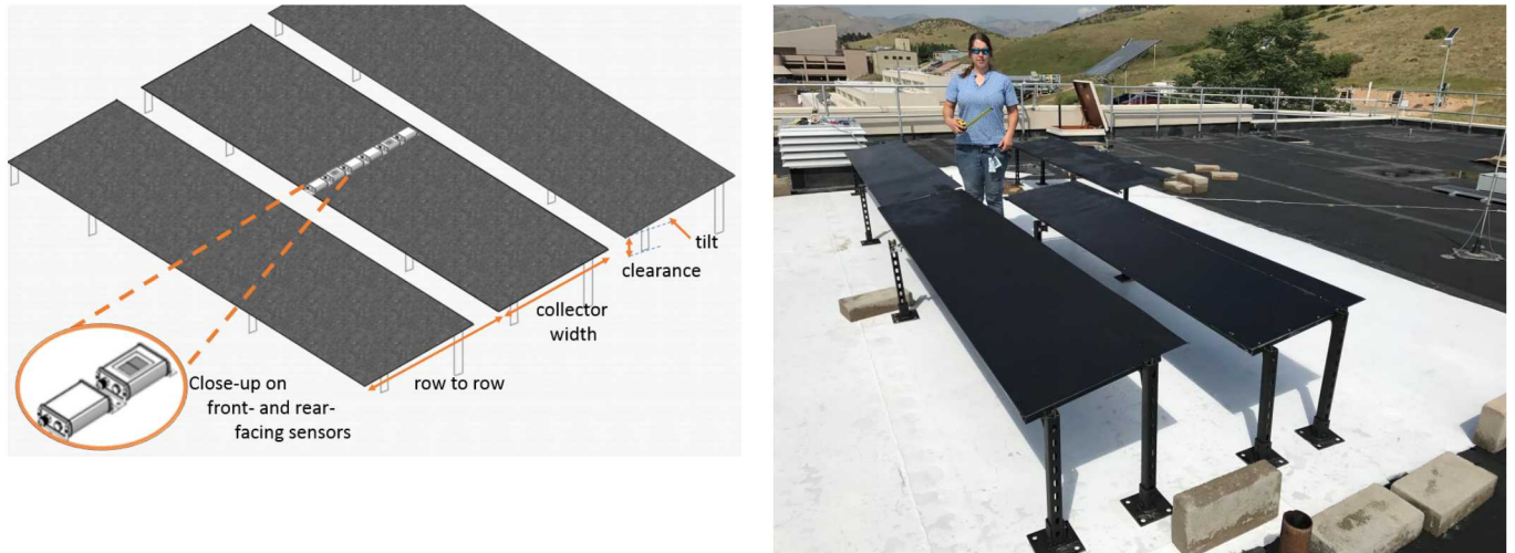
Fig. 12. Diagram (left) of the field test-bed built in Golden, CO, with two front-facing and four back-facing irradiance sensors. The array can be modified for row-to-row spacing, tilt angle, and clearance height. Photograph (right) shows array under construction, ballasts, and the white roof coating. (Ayala et al, JPV 2018)
