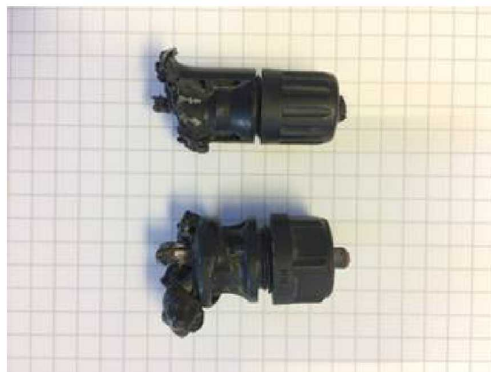
Figure 1. Example of a failed connector retrieved from the field.
