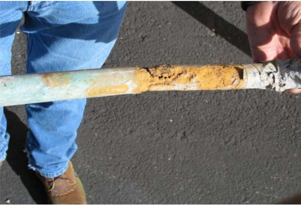
Figure 10. NM Severely corroded steel gas pipe
