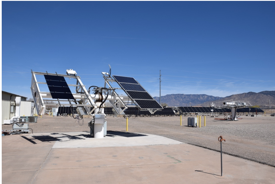
Figure 2-1. Test Devices mounted on two-axis solar tracker
