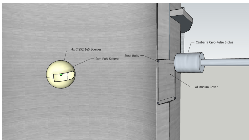
Figure 1 – Illustration of the HDPE moderated Cf-252 source positioned inside the H-Gear
