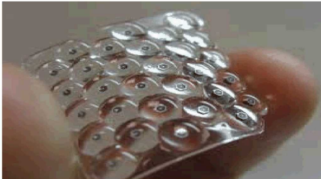
Figure 9: Each PV in this sheet is 300um (Source: Sandia National Laboratories)
