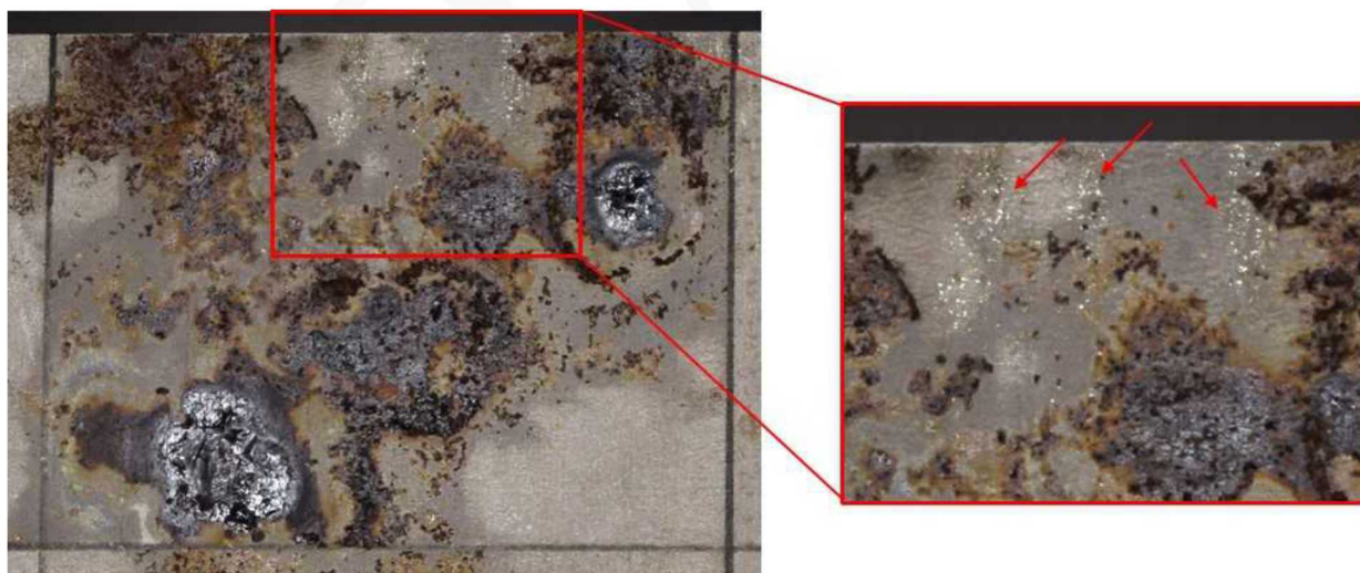
Figure 20. White residue surrounding corroded areas in Quadrant 1 of the 4-point bend specimen.
