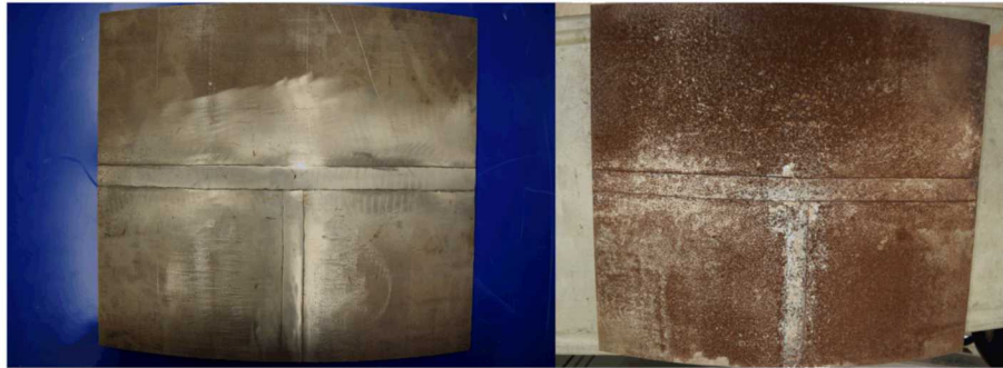
Figure 40. Mock-up plate section as it looked (a) before, and (b) after, \text{MgCl}_2 loading and exposure to 80^\circ\text{C} , 35% RH for 2 months.
