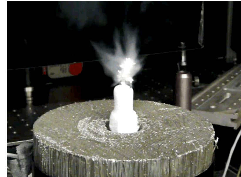
(air, moisture?) icing around liq. H 2 jet column
