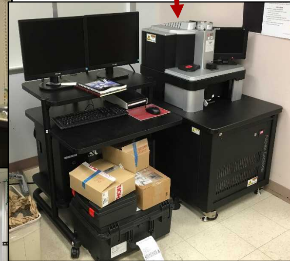
Aspex Explorer SEM-based powder particle analyzer
