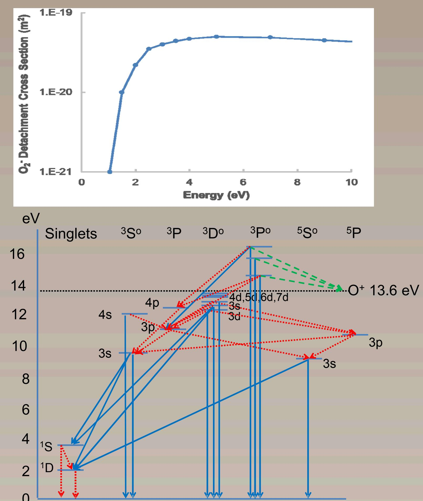
Modeled energy level and transition diagram for atomic O (3D<sup>0</sup>) transitions omitted for clarity). Solid blue lines represent radiative decay in which simulation photons are generated. Red dotted lines represent decay in which a simulation photon is not generated. Green dashed lines are auto-ionizing states.
