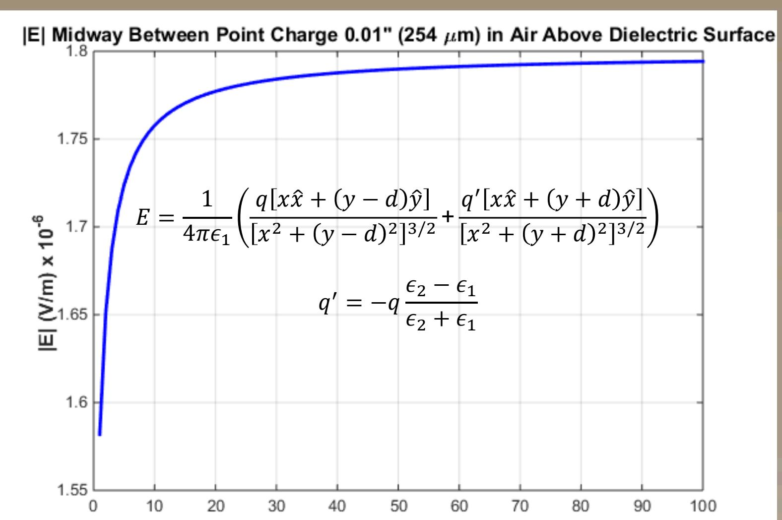
Applying image charge theory, total E-field due to elementary point charge above a dielectric plane modeled as a superpositioning of fields from source and its image within dielectric
