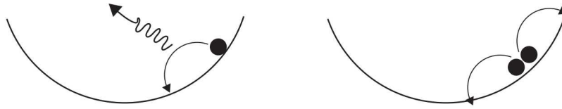
FIGURE 48.12 Conceptual sketch of carrier scattering processes. Left: carrier–phonon interaction, right: carrier–carrier Coulomb interaction.
