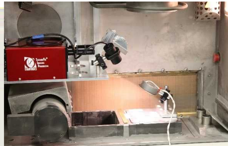
ThermaViz installed in the ProX 200
