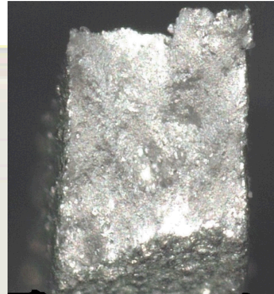
B2, fracture surface optical image by structured light scanning
