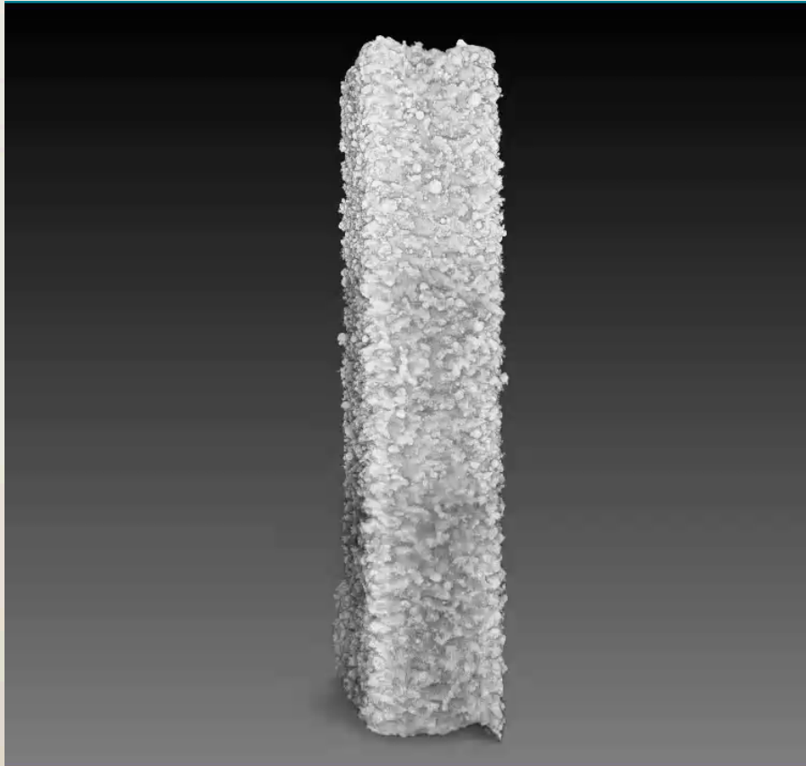
captured defect holes part CT image, Zeiss Xradia Versa voxel resolution \sim 2\mu\text{m}
